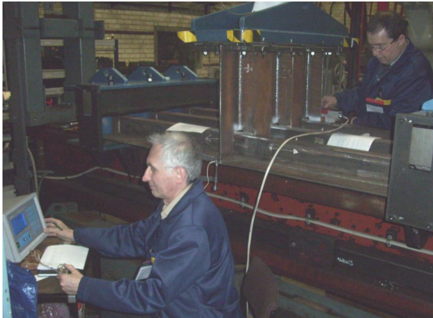
Fig.7. Measurement of residual stresses using UltraMARS system in large-scale welded panel in as-welded condition and during the fatigue loading of the panel
