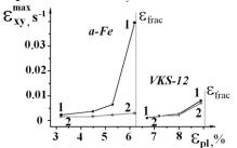
Fig. 1. Changes in the value  $\varepsilon_{xy}$  in macrobands 1 and 2 of ultrafine grain  $\alpha$ -Fe (asymmetric neck) and steel VKS-12 (symmetric neck)
