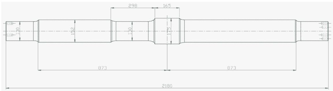
**Figure 6: Full scale cold-rolled specimen specially designed for the crack propagation test**
