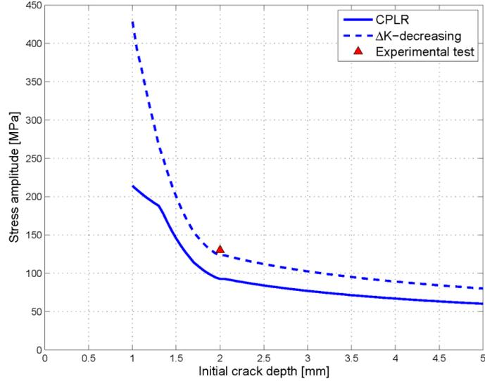
**Figure 4: Minimum stress amplitude of the loading step required for overtaking the threshold SIF**
