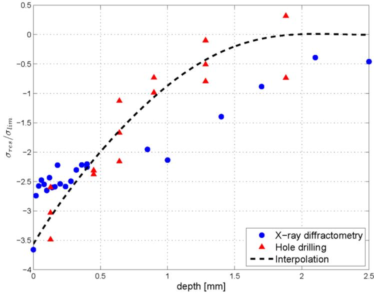
**Figure 3: Longitudinal residual stresses behaviour in depth due to the cold-rolling procedure**
