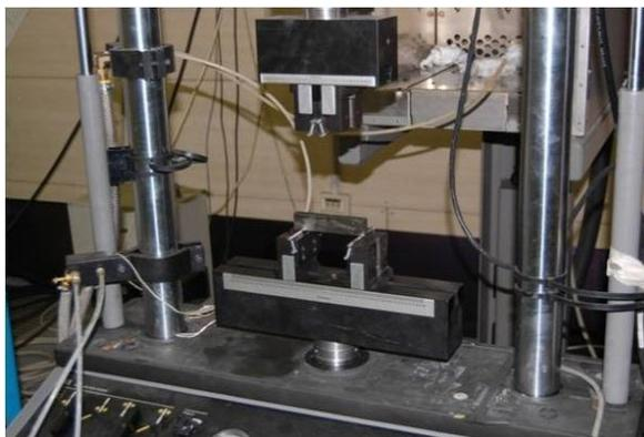
(a) Compression pre-cracking setup
