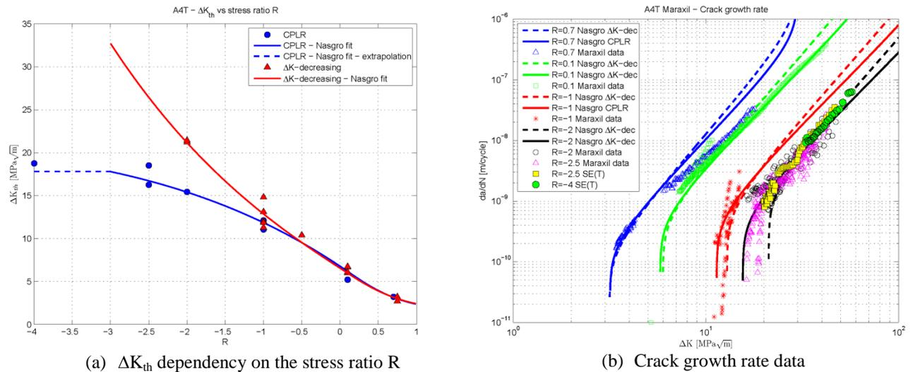
Figure 2: EA4T characterization for crack propagation
