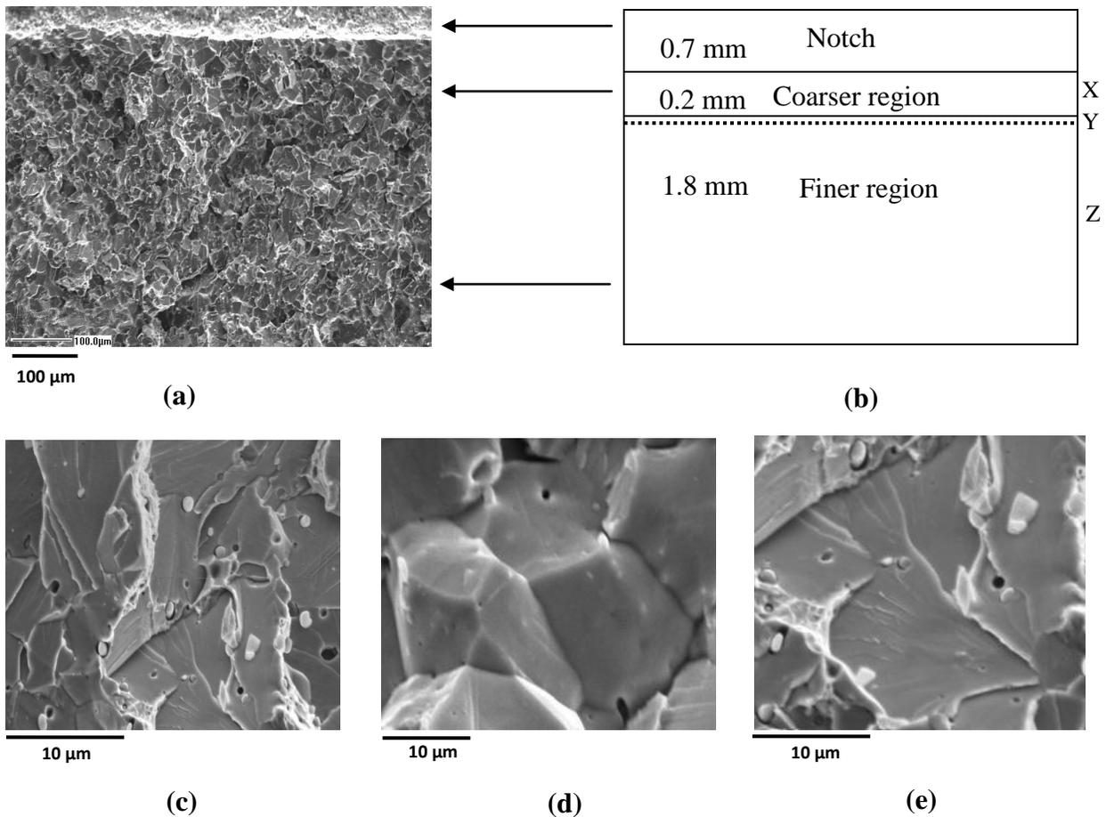
**Figure 3.** (a) Secondary electron image of the fracture surface across the section of the specimen (b) the corresponding schematic diagram showing the related dimensions (c) the coarser grain size region X (d) the localized region Y and (e) the finer grain size region Z
