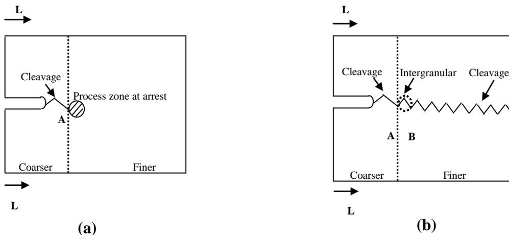
**Figure 4.** A schematic diagram summarizing the crack propagation sequence from the notch root (a) cleavage fracture in the coarser grains up to the coarser to finer interface (b) extension through the process zone and then to final specimen separation
