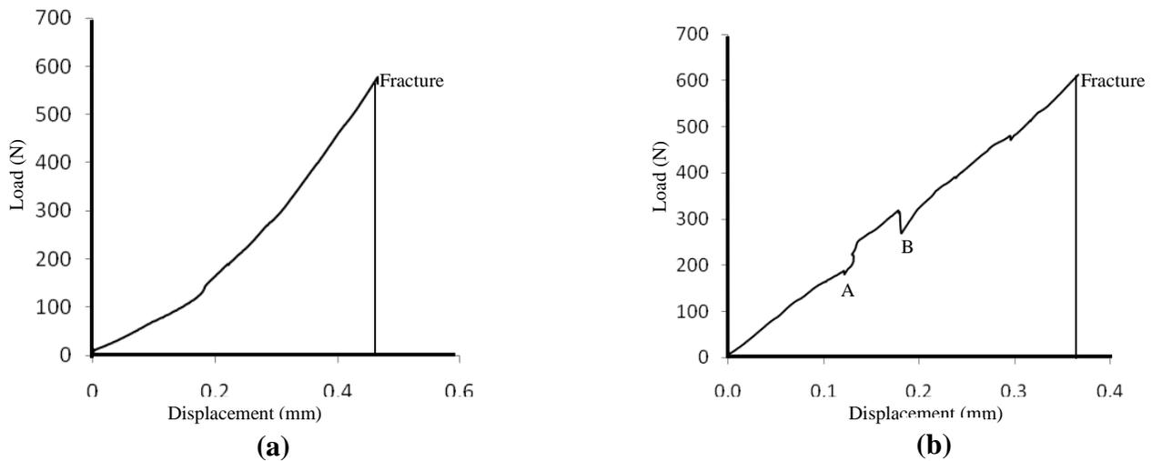
**Figure 2.** The load-displacement curves for the crack growing from (a) finer to coarser grains (b) the coarser to finer grains. The latter shows distinct positions A and B where crack arrest occurs.
