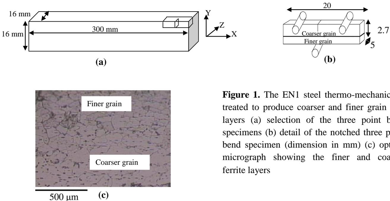
**Figure 1.** The EN1 steel thermo-mechanically treated to produce coarser and finer grain size layers (a) selection of the three point bend specimens (b) detail of the notched three point bend specimen (dimension in mm) (c) optical micrograph showing the finer and coarser ferrite layers
