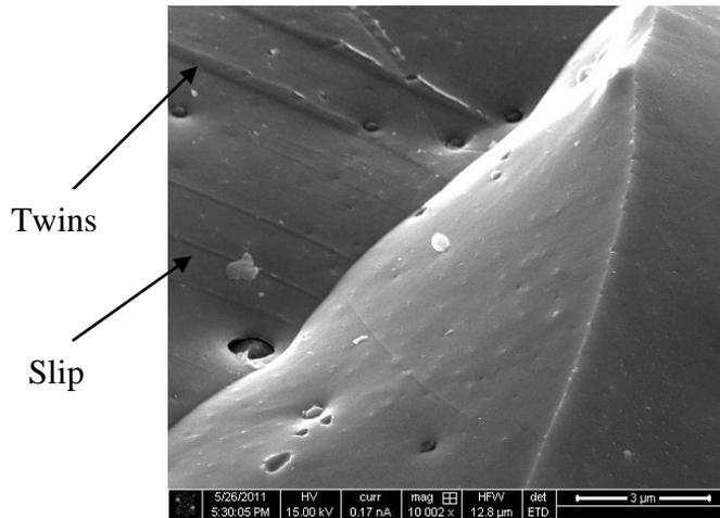
**Figure 5.** A scanning electron micrograph showing the residual damage at the interface between coarser and finer grain region
