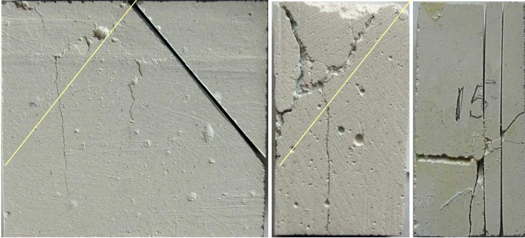
Fig. 4. The sample with the angle of the cuts inclination -  $40^\circ$ . The sample view after testing. Location of the cut axis is shown. At the center – the sample section near the shear front. To the right – the sample side after preparation
