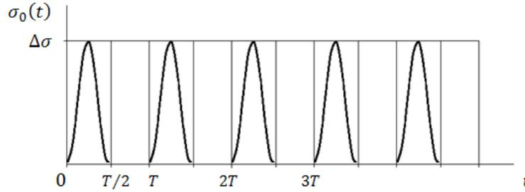
Fig 2. Temporal shape of external loading
