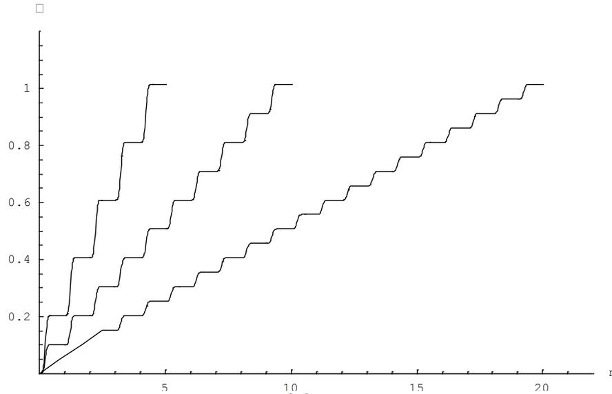
Fig. 3. Microdamage accumulation  $\eta(n)$  under dynamic pulsed loading in 2024-T3 for different load cycling periods (from left to right:  $T = 2\mu s$ ,  $T = 4\mu s$ ,  $T = 8\mu s$ )
