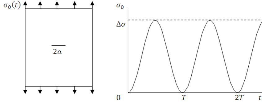
Fig. 1. Fatigue test arrangement
