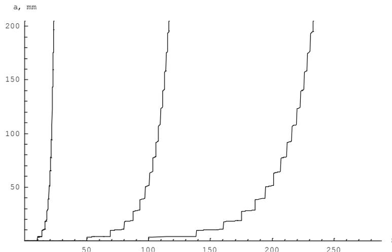
Fig. 4. Crack increment  $a(n)$  under dynamic pulsed loading in 2024-T3 for different load cycling periods (from left to right:  $T = 4\mu s$ ,  $T = 0.2\mu s$ ,  $T = 0.4\mu s$ )
