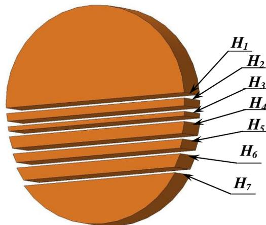
Figure 3 – Scheme of cutting of sample for metallographic study
