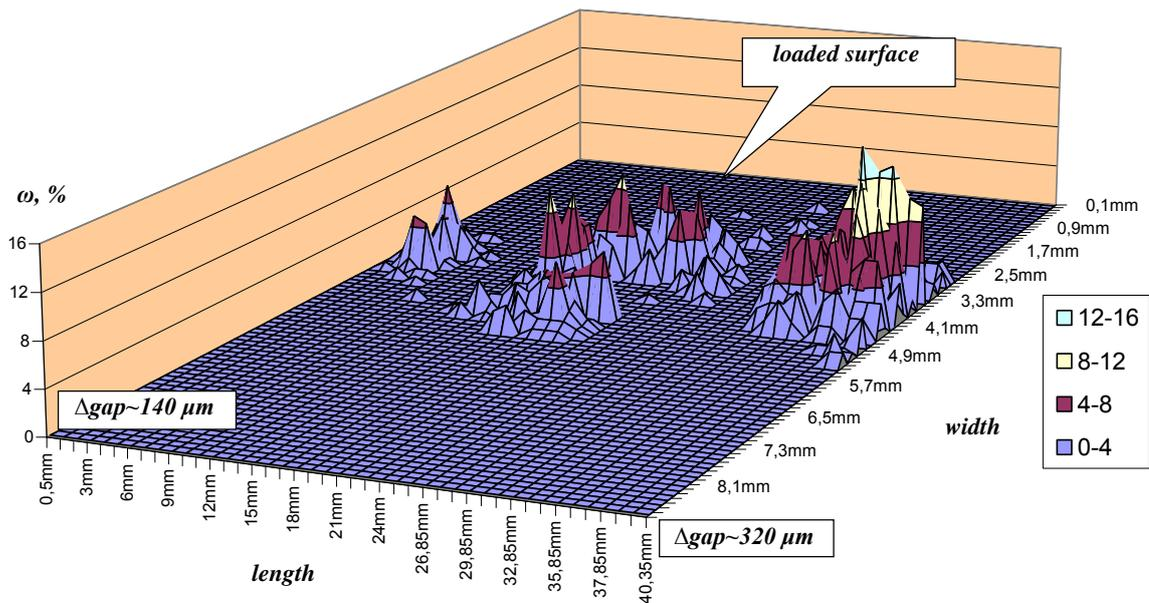
Figure 6 – Damage distribution in the plane of a transverse metallographic section of sample №1 at the depth of the cut  $H_1 \approx 0$  mm
