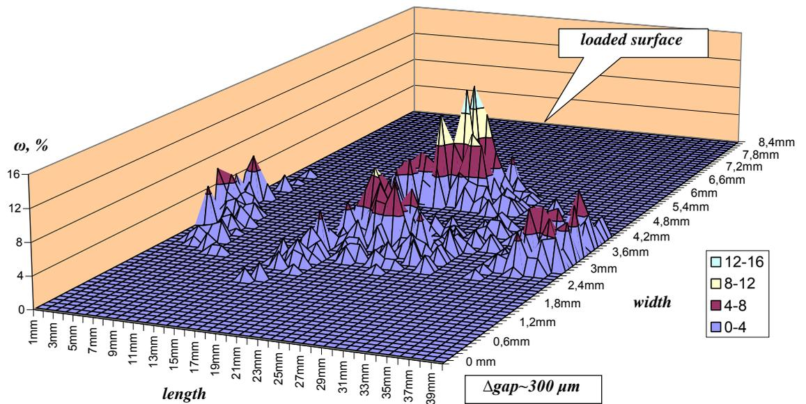
Figure 7 - Damage distribution in the plane of a transverse metallographic section of sample №2 at the depth of the cut  $H_1 \approx 0$  mm
