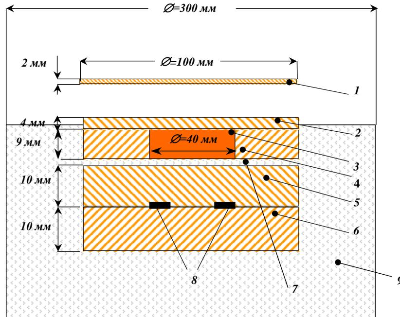
1 – *Cu* liner ( $W_{y0}=1.6 \text{ km/s}$ ); 2 - *Cu* screen; 3 - *Cu* sample; 4 - *Cu* ring;
