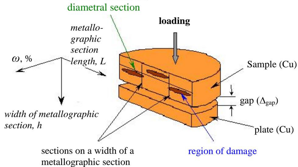
Figure 4 – Schematic image of typical distribution of damage in sample’s cross-section
