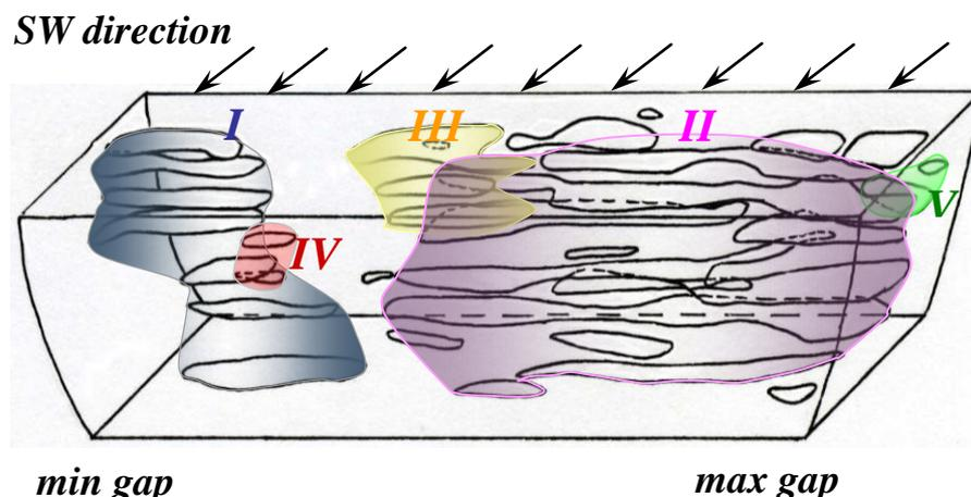
Figure 9 – Space distribution of damage in sample №1. Separate zones are marked by numbers
