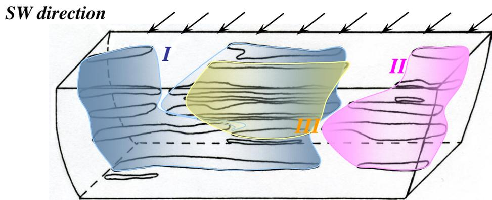
Figure 10– Space distribution of damage in sample № 2. Separate zones are marked by numbers
