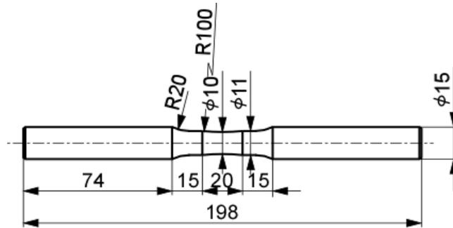
Fig.2. Shape and dimension of the specimen for the fatigue test.
