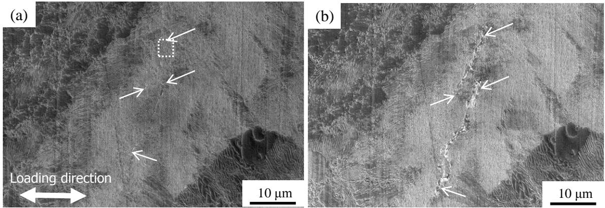
Fig.4. FE-SEM images of the replica around the fatigue crack initiation origin. (Arrows indicate the characteristic points). (a)  $N = 1.0 \times 10^6$  (white line indicates the magnified area of Fig. 7 (a)-(c)). (b)  $N = 1.0 \times 10^7$ .
