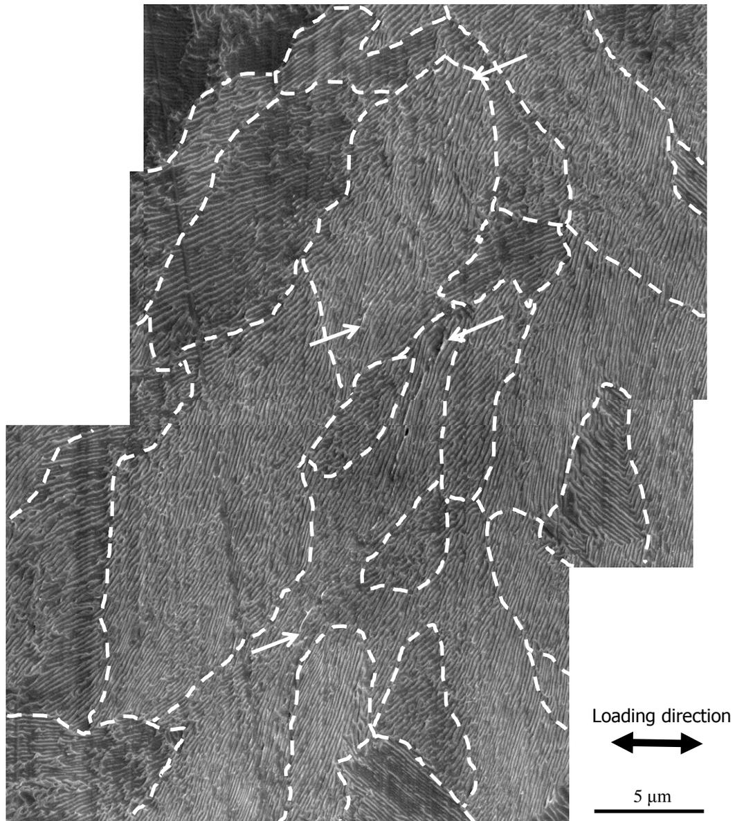
Fig.7. Relation between crack initiation and domain of the pearlite colony (dashed white lines indicate the boundaries of the pearlite colonies, arrows indicate the crack tips).
