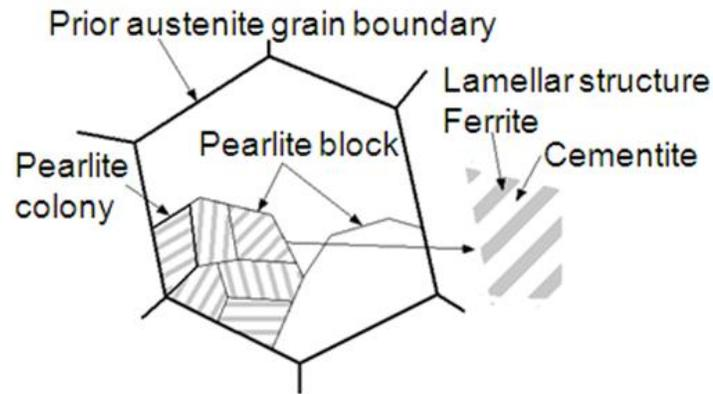
Fig.1. Schematic diagram of pearlitic steel microstructure.
