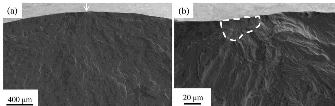
Fig.3. SEM images of the fracture surface and fatigue crack initiation origin. (a) Around the fatigue crack initiation origin. (b) Magnification of (a); dashed line shows the boundary of the fatigue crack initiation origin domain.
