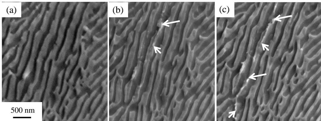
Fig.6. FE-SEM images of the replica around the fatigue crack initiation origin. (Arrows indicate the characteristic points). (a)  $N = 0$ . (b)  $N = 1.0 \times 10^4$ . (c)  $N = 1.0 \times 10^6$ .
