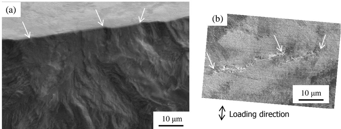
Fig.5. Around the fatigue crack initiation origin (arrows indicate the characteristic points). (a) Fracture surface and surface of the fractured specimen. (b) Replica (mirror-reversed image,  $N = 1.0 \times 10^7$ )
