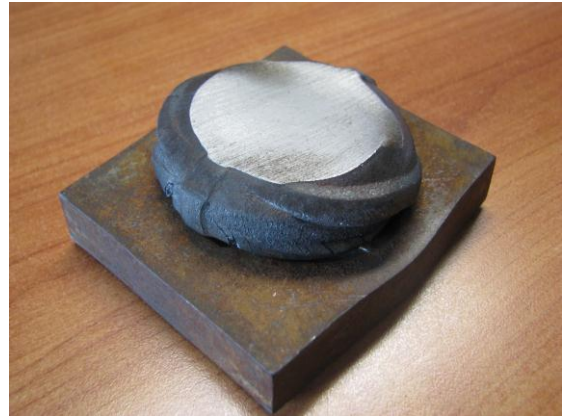
Figure 11: (a) Experimental set-up for the compressive test performed on specimen S_2 using the Galdabini hydraulic press. The \text{He}^3 neutron detector has been placed at a distance of about 10 cm from the monitored specimen. (b) Specimen S_2 at the end of the test.
