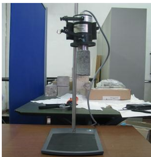
Fig. 7. The Luserna stone specimen connected to the ultrasonic horn. The ultrasonic apparatus (Bandelin HD 2200) consists of a generator that converts electrical energy to 20 kHz ultrasound, and of a transducer that switches this energy into mechanical longitudinal vibration of the same frequency.
