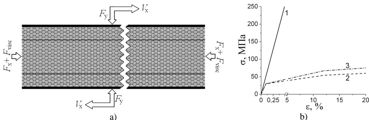
Fig. 1. a) structure and loading scheme of simulated specimen; b) response functions of automata of blocks (1), interfaces in inner part of specimen (2) and on surface layers (3). Wavy line in the figure (a) schematically indicated by a conventional line break.
