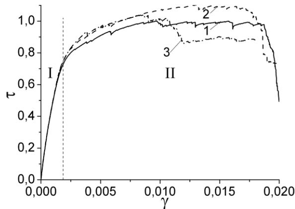
Fig. 3. Graphs of dependences of shear resistance force of simulated system ( $\tau$ ) on value of shear strain ( $\gamma$ ): 1 -  $C_\sigma=0$ ; 2 -  $C_\sigma=0,5$ ; 3 -  $C_\sigma=1$ . Roman numerals I and II denotes quasielastic and quasiplastic stages of loading diagrams.
