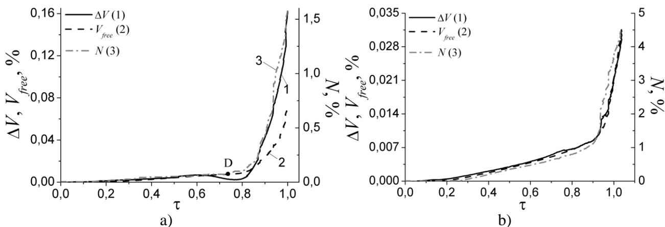
Fig. 6. Graphs of dependences of volume changing ( $\Delta V$ ), free volume ( $V_{free}$ ) and number of damages ( $N$ ) on value of shear stress  $\tau$ . a)  $C_\sigma = 0$ ; b)  $C_\sigma = 1$ .
