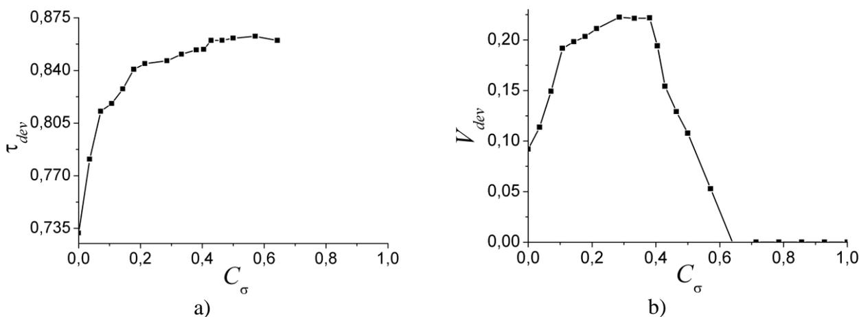
Fig. 7. Graphs of dependences of the specific force of resistance to shear deformation at the time of activation of the shear slip (a) and the value of the difference between the ultimate values of the total change of the volume and free volume (b) on the parameter  $C_\sigma$ .
