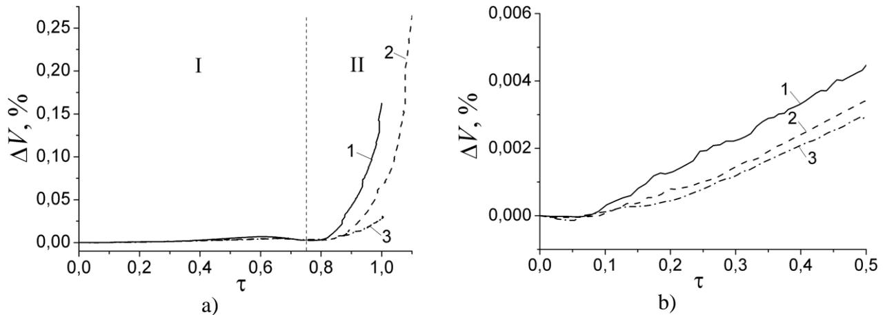
Fig. 2. Graphs of dependences of relative changing of the volume of the specimen  $\Delta V$  on shear stress level  $\tau$ : 1 -  $C_\sigma=0$ ; 2 -  $C_\sigma=0,5$ ; 3 -  $C_\sigma=1$ . In figure (a) is shown extended range of shear stresses  $\tau \in [0, 1]$ , in the figure (b) initial interval  $\tau \in [0, 0,5]$  Curves 1-3 in figure (a) are shown up to the moment of achievement of ultimate state of the system (maximum value of  $\tau$ ).
