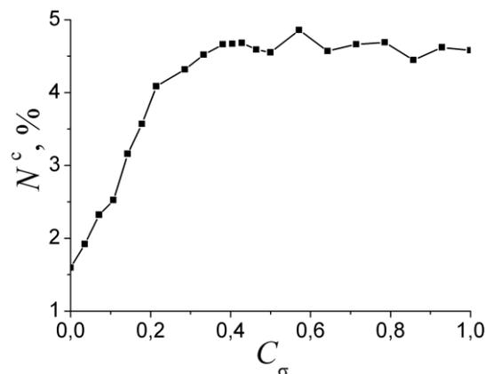
Fig. 5. Graph of dependence of value of accumulated damages  $N^c$  to the moment of achieving of ultimate state of the specimen on the parameter  $C_\sigma$ .
