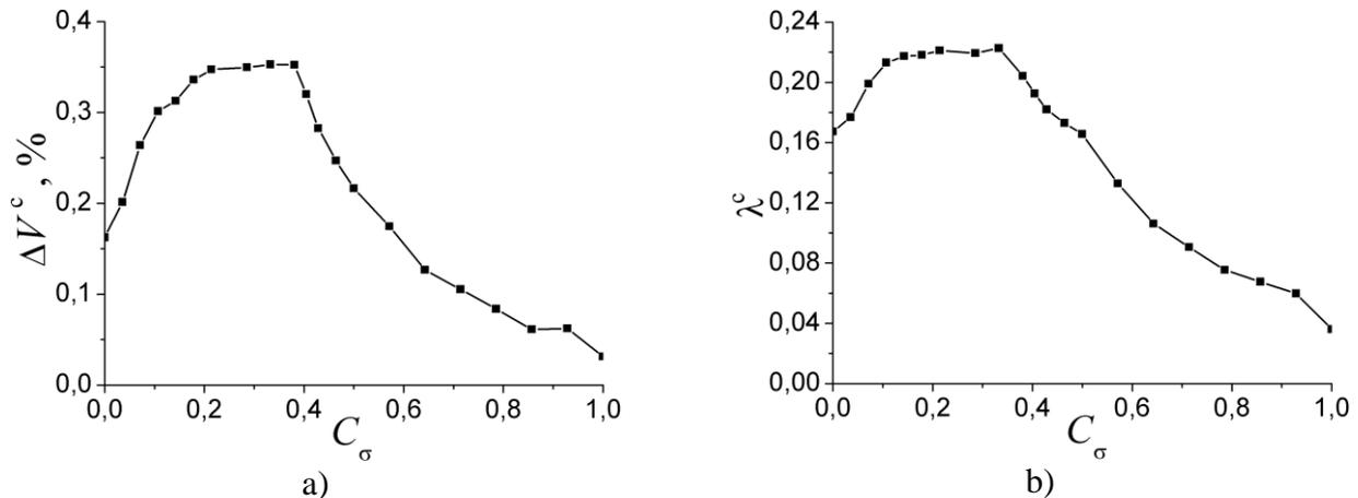
Fig. 4. Graphs of dependences of relative changing of volume of the specimen  $\Delta V^c$  (a) and dilatancy coefficient  $\lambda^c$  (b) to the moment of reaching of ultimate state of the system on parameter  $C_\sigma$ .
