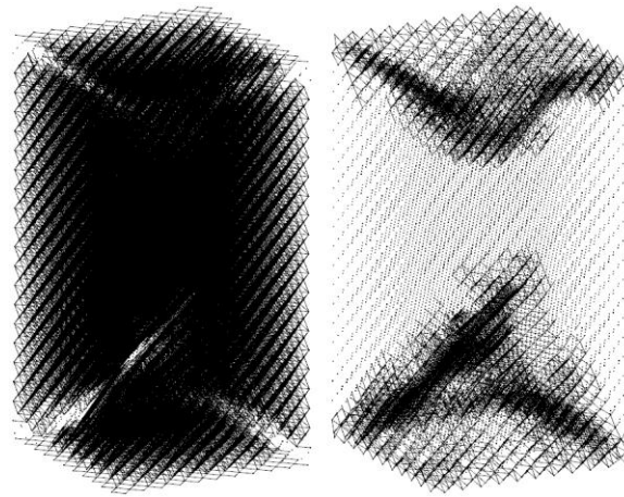
Fig.2. Fracture pattern of a solid ceramic specimen under compression: a) lines connect linked automata, b) lines connect unlinked automata.
