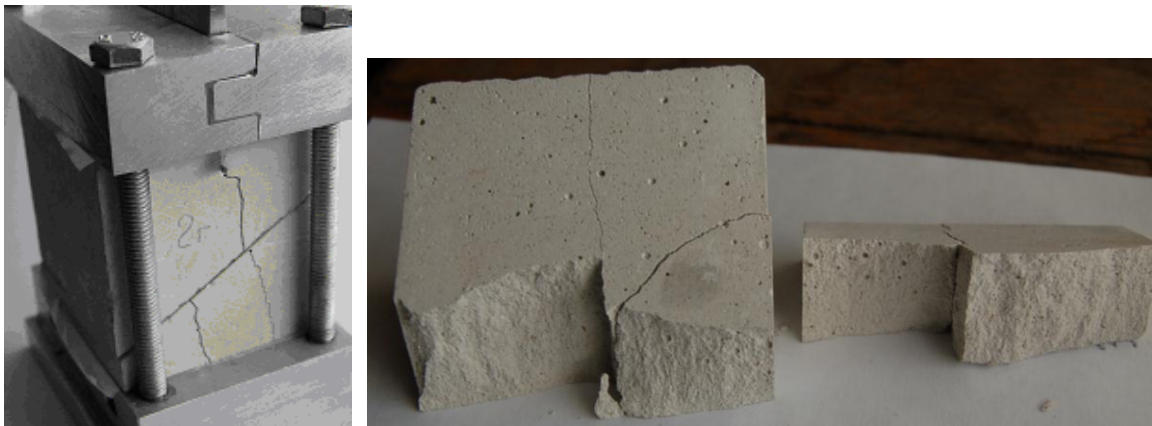
Fig. 7. Sample after testing. Secondary cracks - to the right ( \alpha = 30^{\circ} , \sigma = 0.45 MPa)
