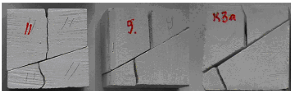
Fig. 8. Samples after testing. An increase of the size d of the slipping zone at increasing the angle \alpha of the interface plane inclination is seen
