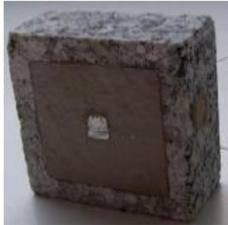
Fig.4. The rock sample of granite with an electric contact on the sample fixed by DiAg paste
