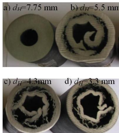
Fig.2 Sections after implosion by HE GH-920 with different HE thickness of  $d_H$
