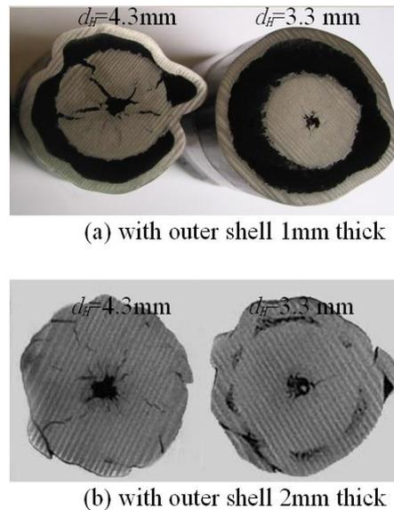
Fig.3 Sections of steel tube after sliding implosion by HE GH-925 with an shield shell ( $d_H$  --HE thickness)
