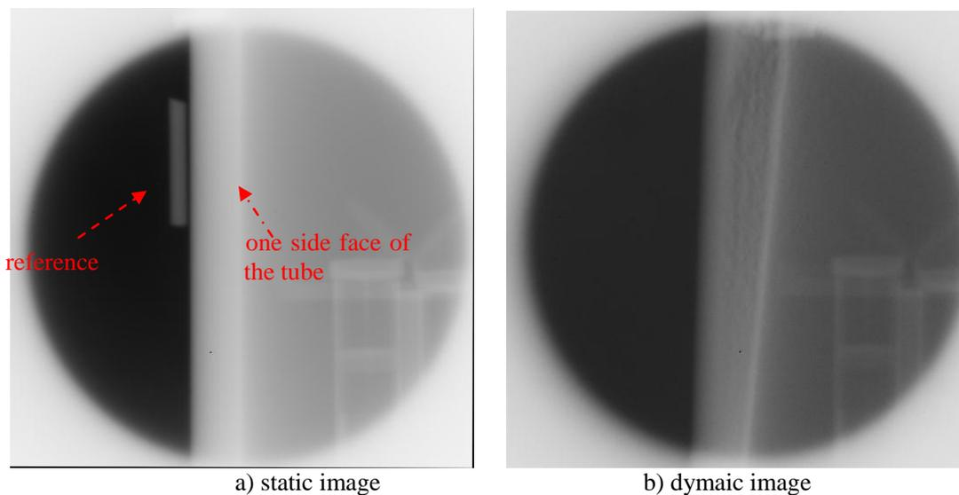
Fig.5 The flash-radiography image of the OFHC copper tube
