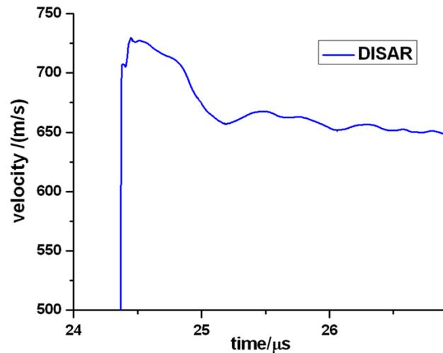
Fig.4 Inner-surface velocity profile of OFHC copper tube
