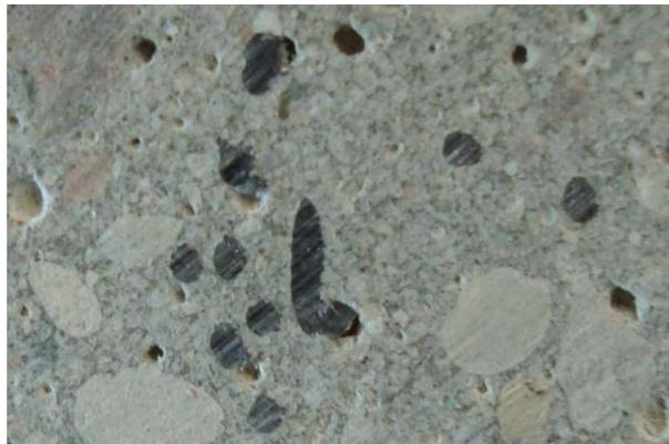
Fig. 2. Micrograph of the specimen's cross-section showing fibers distribution and orientation.
