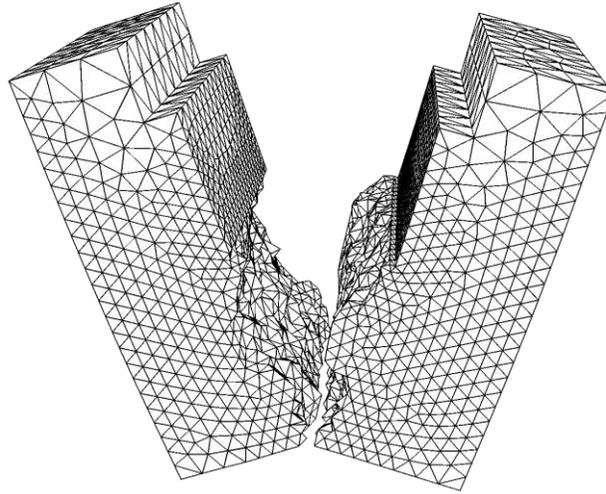
Fig.6. Finite element simulation of wedge splitting test.
