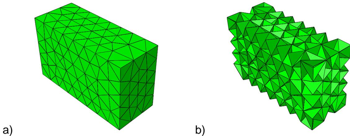
Fig.5. Original 3D finite element mesh (a) and cohesive elements embedded between all solid elements (b).
