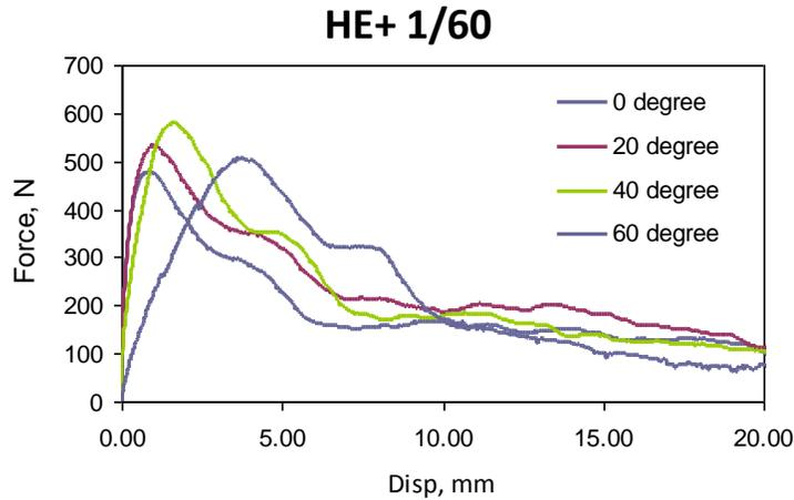
Fig. 1 Pull-out behavior of HE+ 1/60 hook-end steel fibers embedded at different angles.
