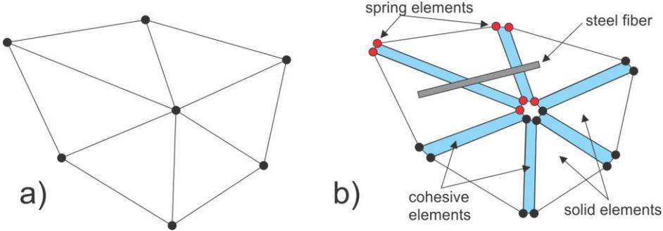
Fig.4. Original finite element mesh (a) and modified mesh with separated solid elements, embedded cohesive elements and spring elements (b).
