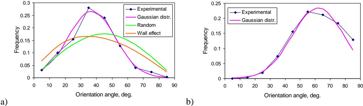
Fig. 3. The theoretical and experimental distribution of angles between the fibers and normal to the fracture plane (a); experimental distribution of angles between the fibers and vertical axis (b).
