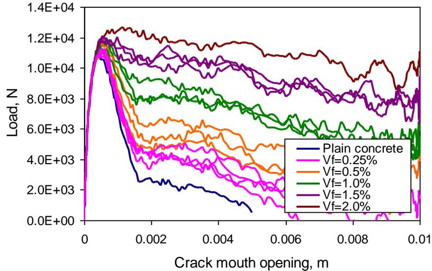
Fig.7. Results of wedge splitting test simulation: load-deflection curves for plain concrete and fiber-reinforced concrete with different fiber volume fractions.
