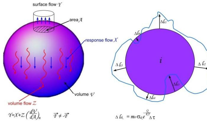
Fig. 5. The scheme of dissipative processes: a) volume and surface flows (G.C. Sih, [6]), b) SECA.
