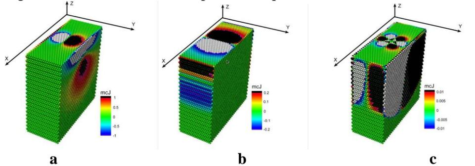
Fig. 3. Distribution of the couple force components: a)  $M_x$ , b)  $M_y$ , c)  $M_z$ .
