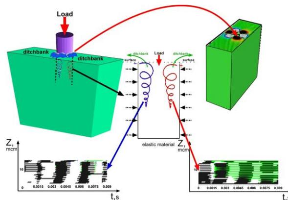
Fig. 4. The scheme of generation of spiral waves under the indenter.
