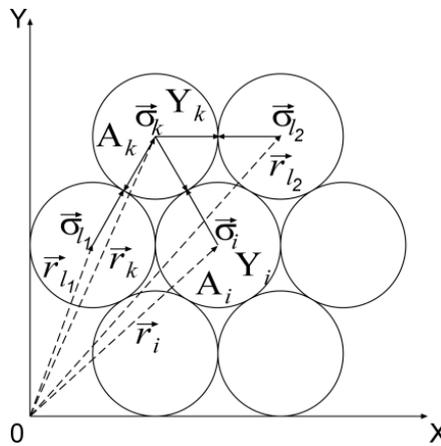
Fig. 1. 2D element of cellular automaton ( $i$ -th) and its first coordination sphere. Schematic picture of calculation of the principal stress and the couple force.
