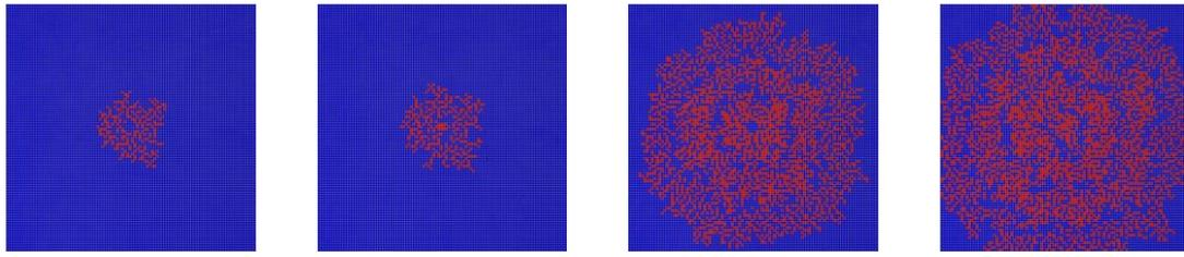
Fig. 8. Simulation of evolution of defect structure at 2D interface under variation of the hidden variables:  $P=0,2$ ;  $L=25$ ;  $D=5$ .
