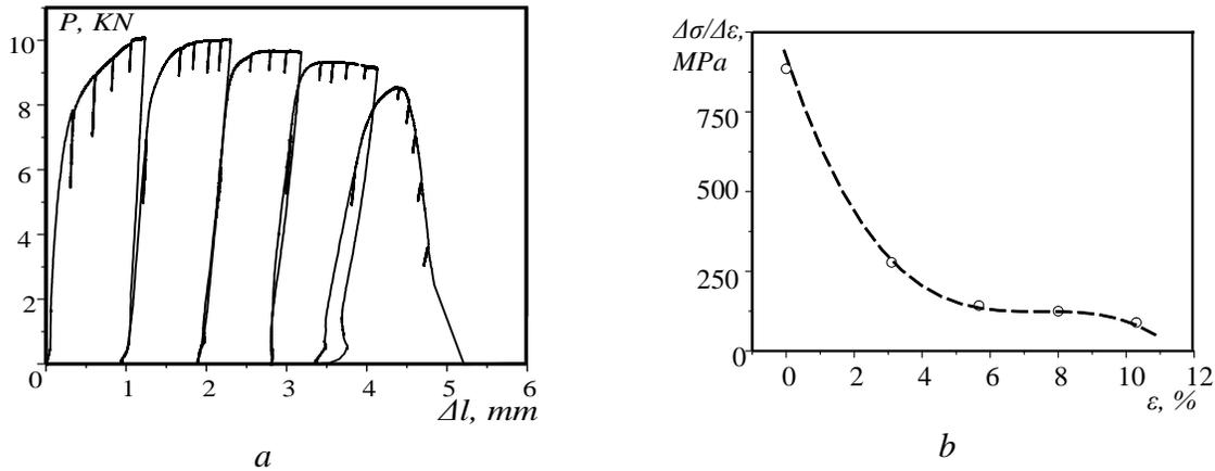
Fig. 5. Stress-strain curve of the material with multiple defects (a) and dependence of variation of the material deformation capacity on the relative strain of the specimen (b)
