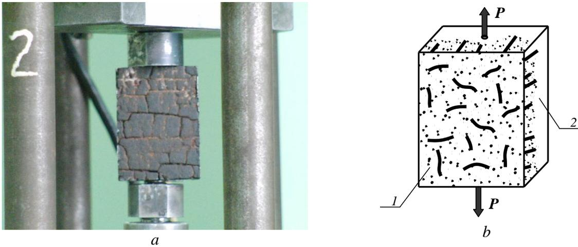
Fig. 1. Scheme of testing the specimen with a network of thermal fatigue cracks: 1 – external layer; 2 – internal layer
