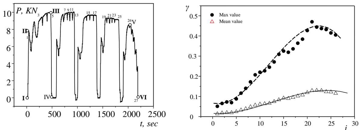
Fig. 2. Dependence of specimen loading  $P$  on duration of deformation  $t$  (a) and shear strain intensity at measurement point  $i$  (b)
