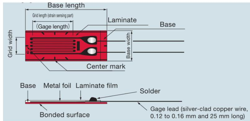
Fig.1 Schematic illustration of strain gage [1].
