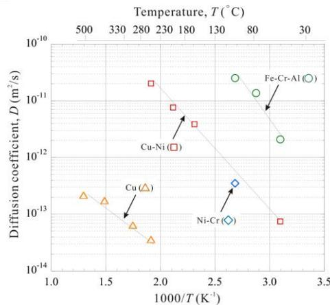
Fig. 5 Arrhenius plot of hydrogen diffusion coefficient of Cu-Ni, Ni-Cr, Fe-Cr-Al and Cu.
