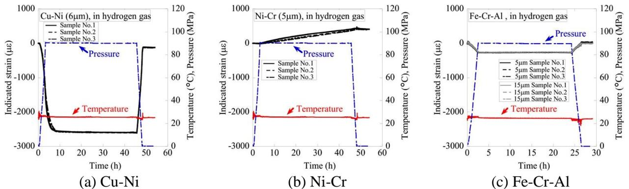
Fig.2 Output of strain gage in 90 MPa hydrogen gas.
