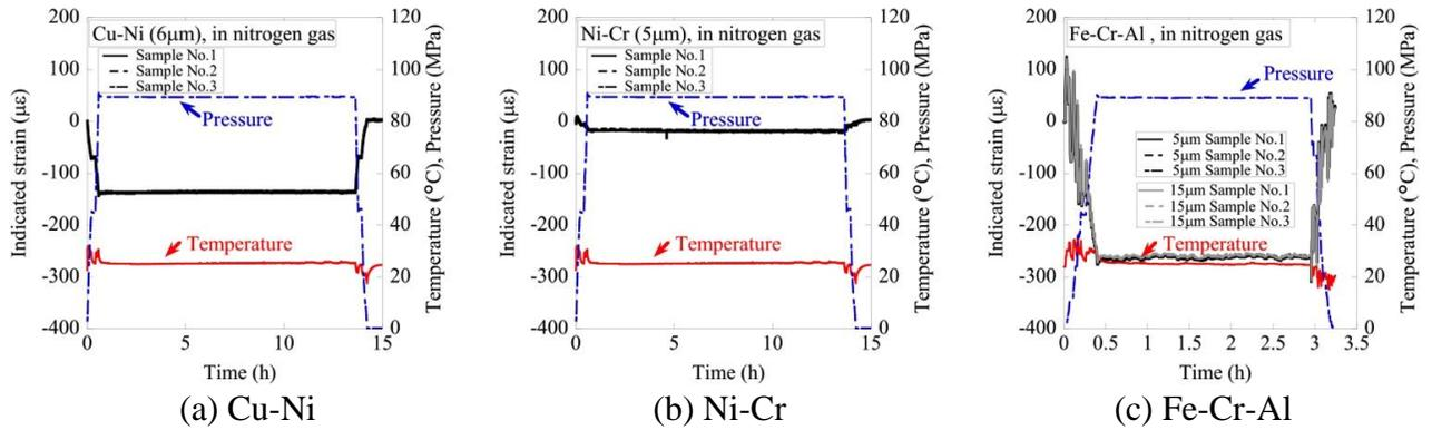
Fig. 3 Output of strain gage in 90 MPa nitrogen gas.
