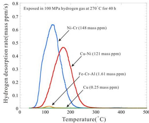
Fig. 4 Hydrogen desorption profiles of Cu-Ni, Ni-Cr, Fe-Cr-Al and Cu exposed in 100 MPa hydrogen gas at 270 °C for 40 h
