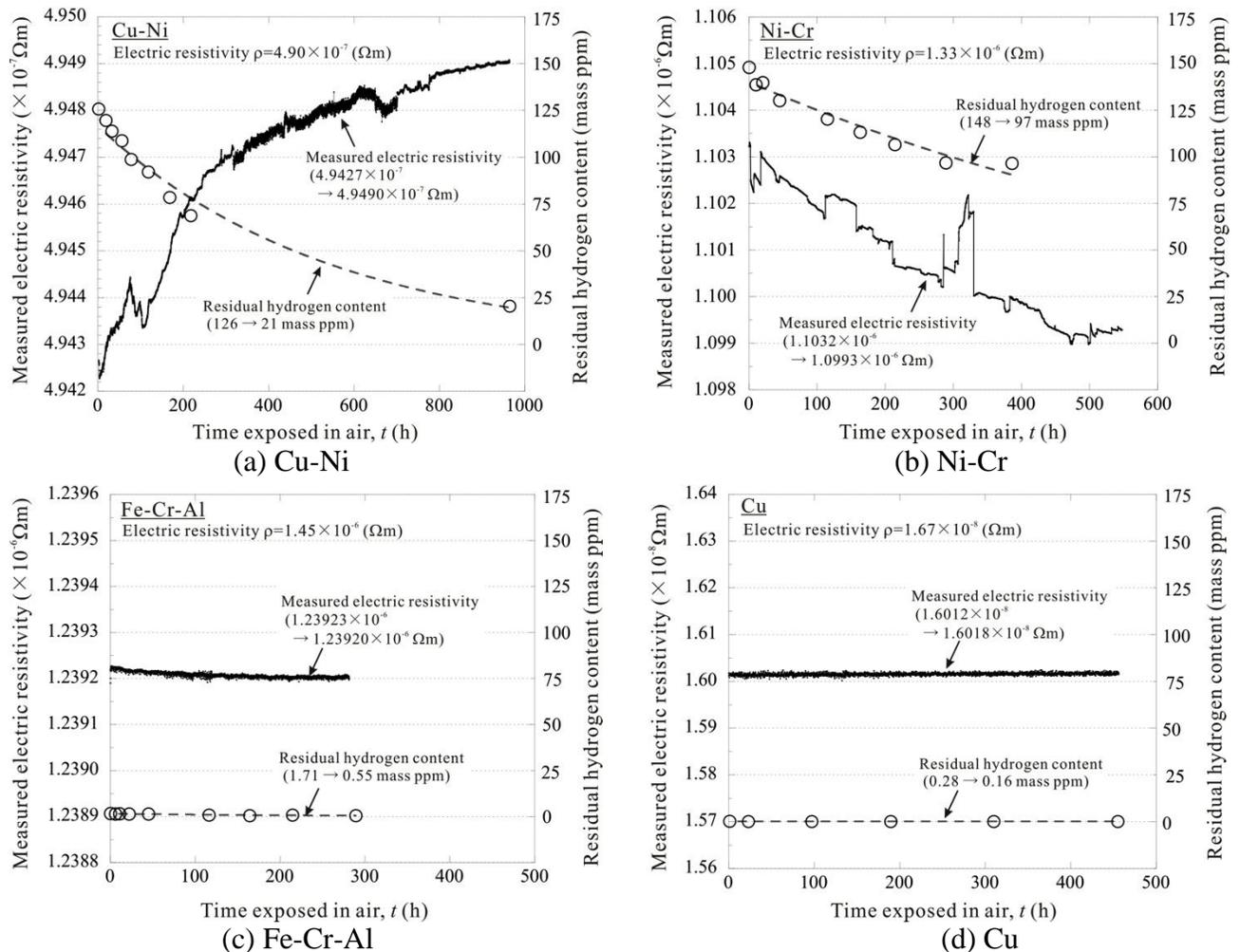
Fig. 6 Relationship between electric resistivity and residual hydrogen content.
