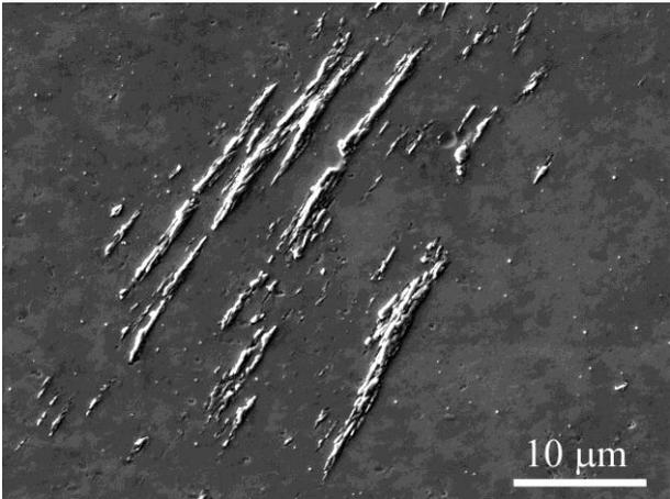
Fig. 3: Cyclic slip bands produced by high-cycle fatigue. The loading axis is horizontal.
