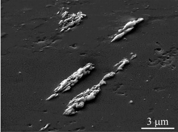
Fig. 1: Cyclic slip bands developed after fatigue loading with  $\sigma_a = 130$  MPa for  $2.3 \times 10^{10}$  cycles.
