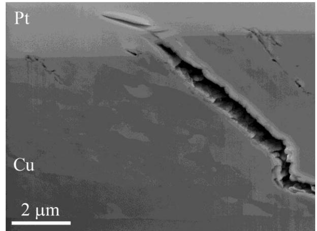
Fig. 8: FIB cut across the fatigue crack perpendicularly to the surface.
