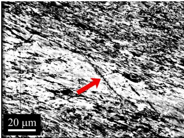
Fig. 7: Fatigue crack and microstructure displayed by means of FIB.
