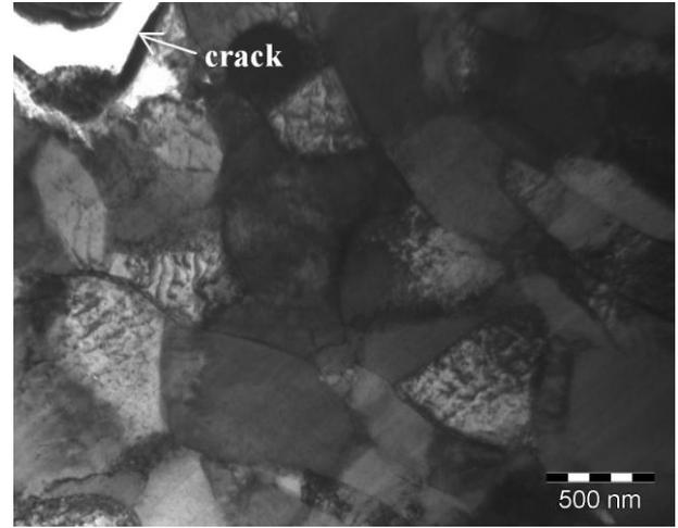
Fig. 11: Thin foil prepared by means of FIB showing the microstructure around fatigue crack. TEM.
