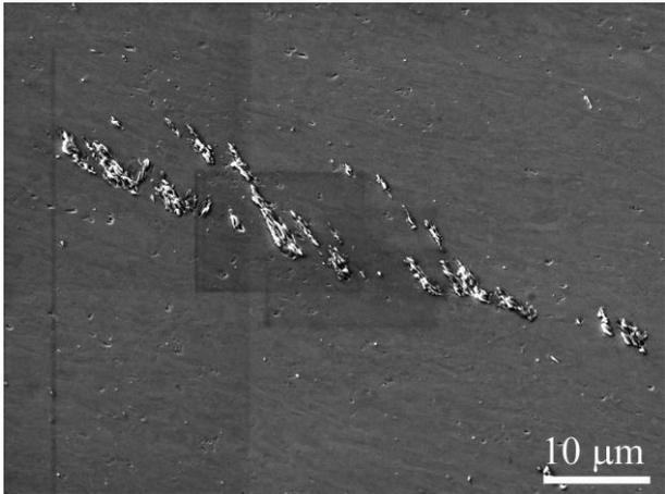
Fig. 4: Cyclic slip bands on the same specimen as in Fig. 3, however turned around the circumference by an angle of  $90^\circ$ .
