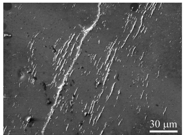
Fig. 6: Surface relief and fatigue crack after  $6.2 \times 10^6$  cycles at the stress amplitude  $\sigma_a = 170$  MPa.
