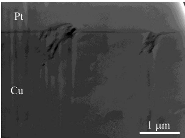
Fig. 9: FIB cut of cyclic slip bands developed during cycling with  $\sigma_a = 170$  MPa.
