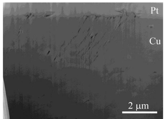
Fig. 10: FIB cut of cyclic slip bands formed after giga-cycle fatigue loading.
