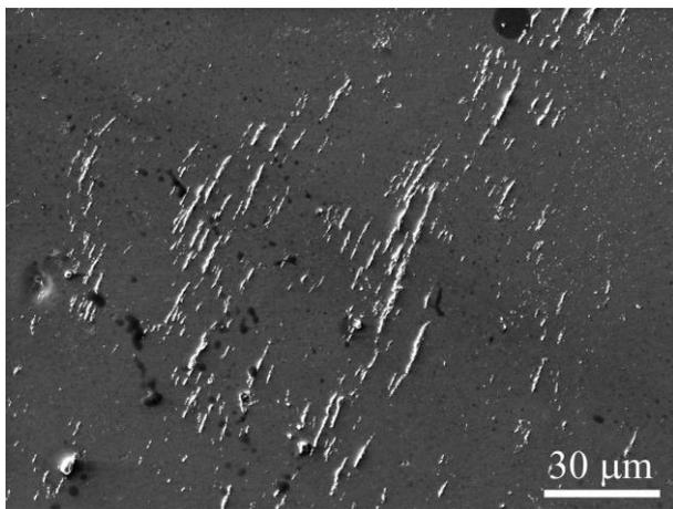
Fig. 5: Surface relief after  $9.5 \times 10^5$  cycles at the stress amplitude  $\sigma_a = 170$  MPa.
