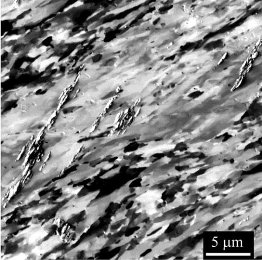
Fig. 2: Cyclic slip bands in the zone of near-by oriented grains after gigacycle fatigue loading.
