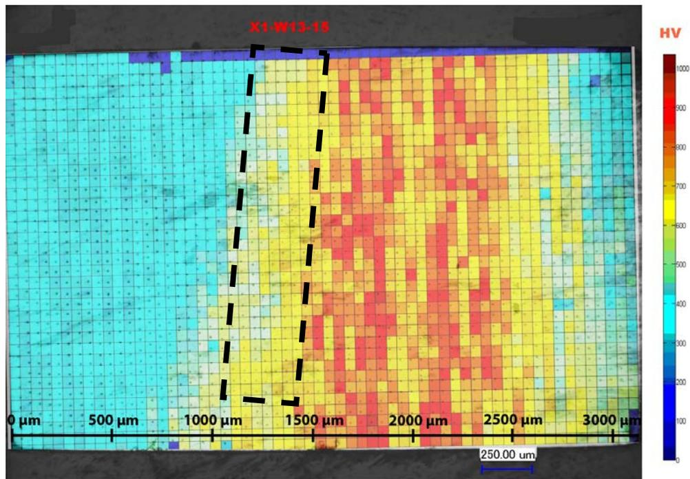
Fig. 6 – Micro-hardness measurement of the fracture surface
