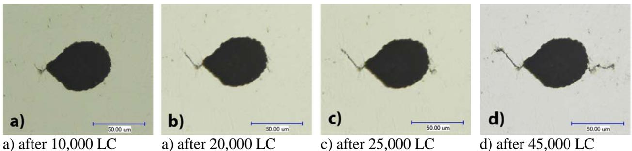
Fig. 9 – Crack growth at the notch tip and backside
