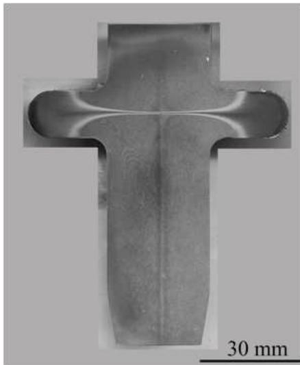
Fig. 1 – Cross-section micrograph of the flange shaft, etched
