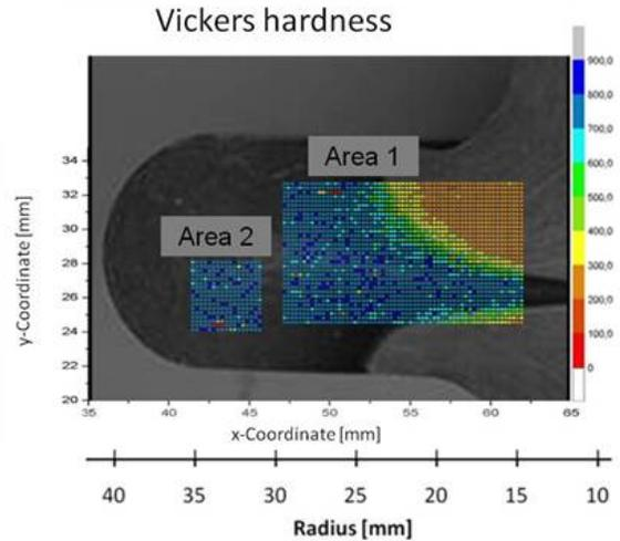
Fig. 2 - Phase distribution identified by using micro-hardness indentation
