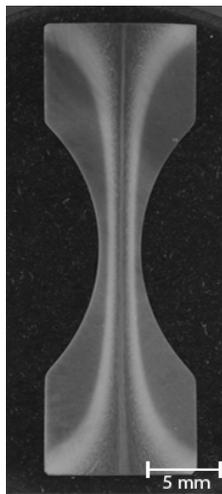
Fig. 3 – micro specimen, polished and etched
