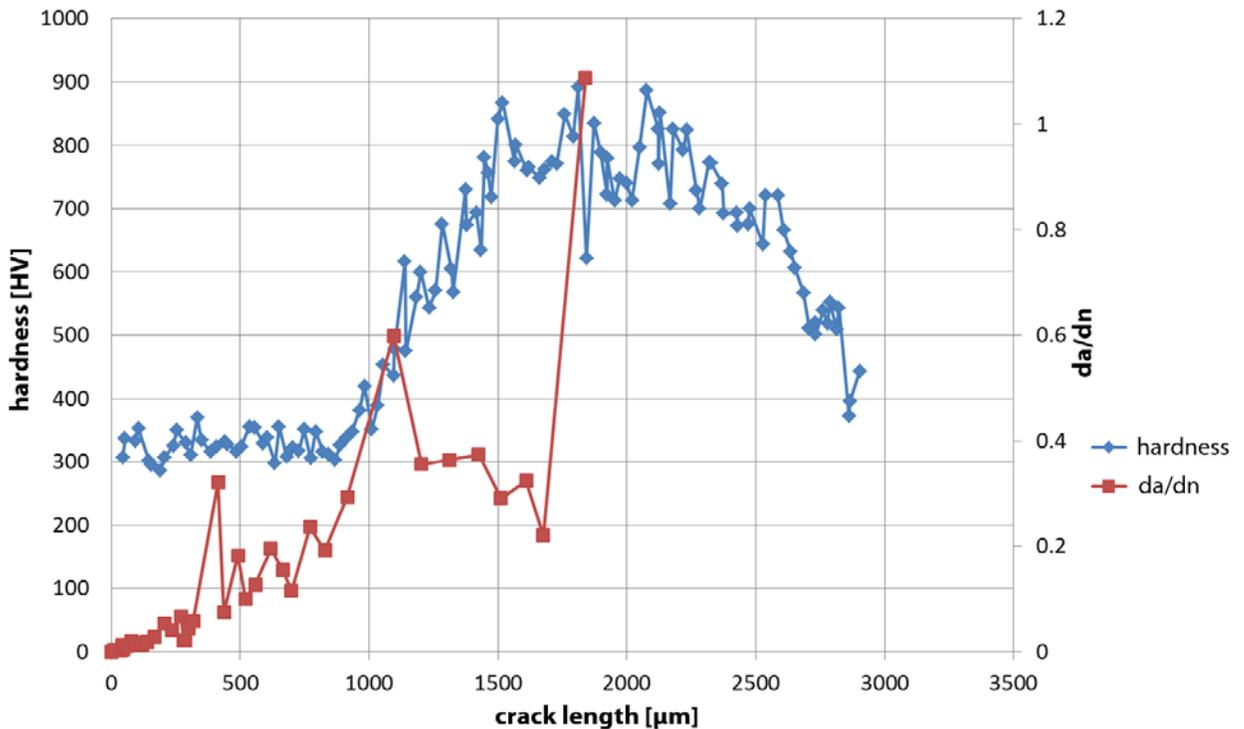
Fig. 7 - Hardness and  $da/dn$ -curve related to the crack length
