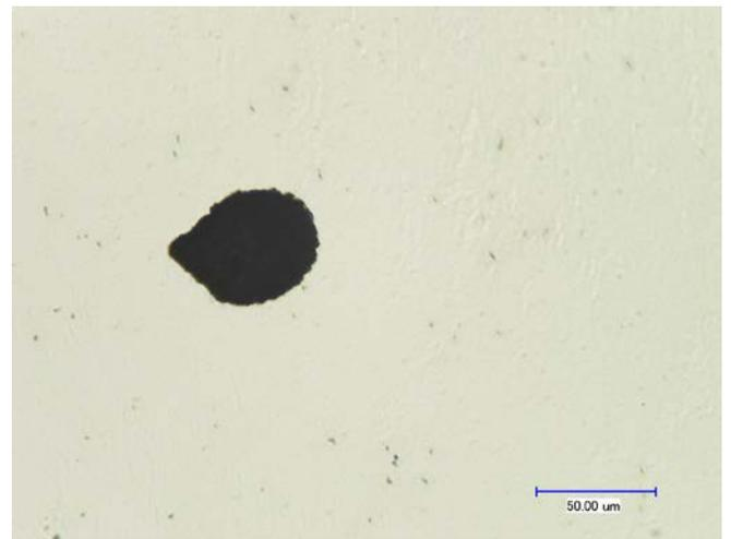
Fig. 4 - Micro-notch manufactured by femtosecond laser ablation
