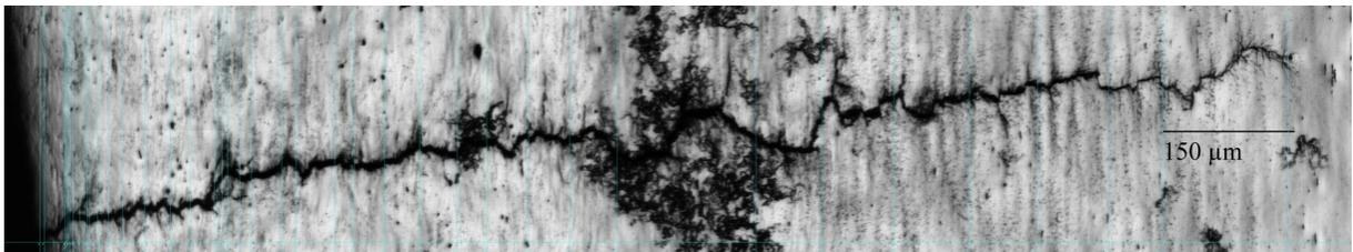
Fig. 5 – Fatigue crack starting from the specimen edge in the ferrite/perlite phase
