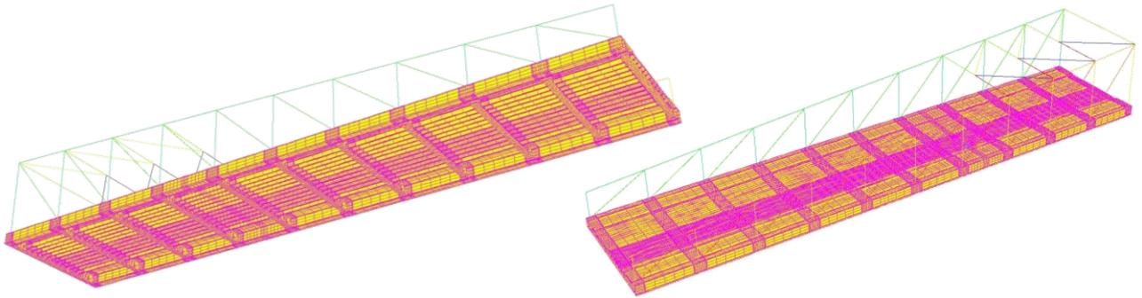
Fig. 7: FEM-model of the Temse bridge
