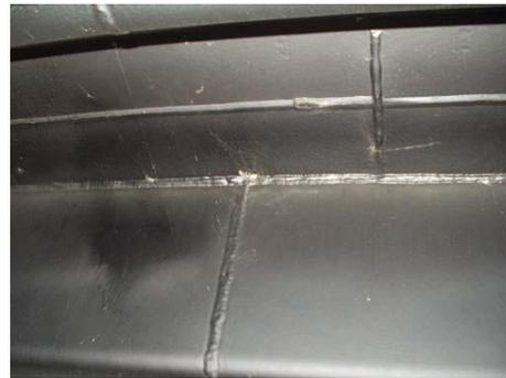
Fig. 6: Multiple welds intersecting at the crack location
