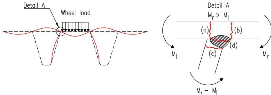
Fig. 3: Schematic deformation under wheel loading and the corresponding crack directions
