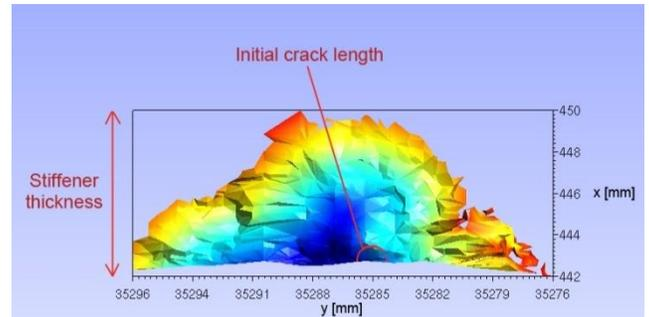
Fig. 11: Crack front dimensions
