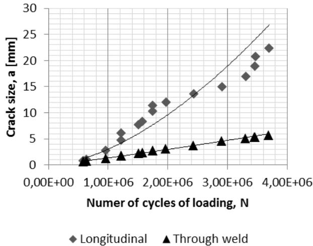
Fig. 10: Comparison of the longitudinal crack propagation and the propagation through the weld
