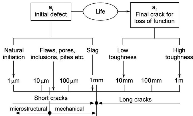
Fig. 1: Length scales of the life cycle of a component subjected to cyclic loading (according to [1])
