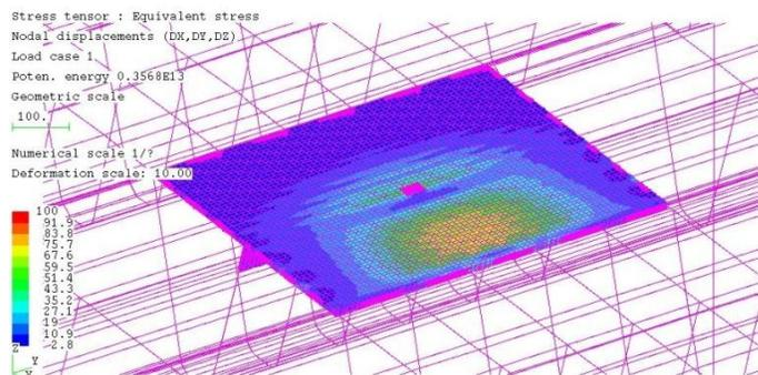
Fig. 8: Stresses in the 3D volume elements for the XFEM calculations due to an axle load of 90 kN
