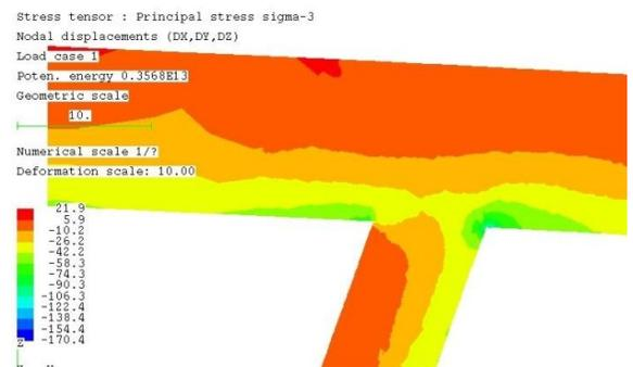
Fig. 9: Stresses in the weld detail without any cracks
