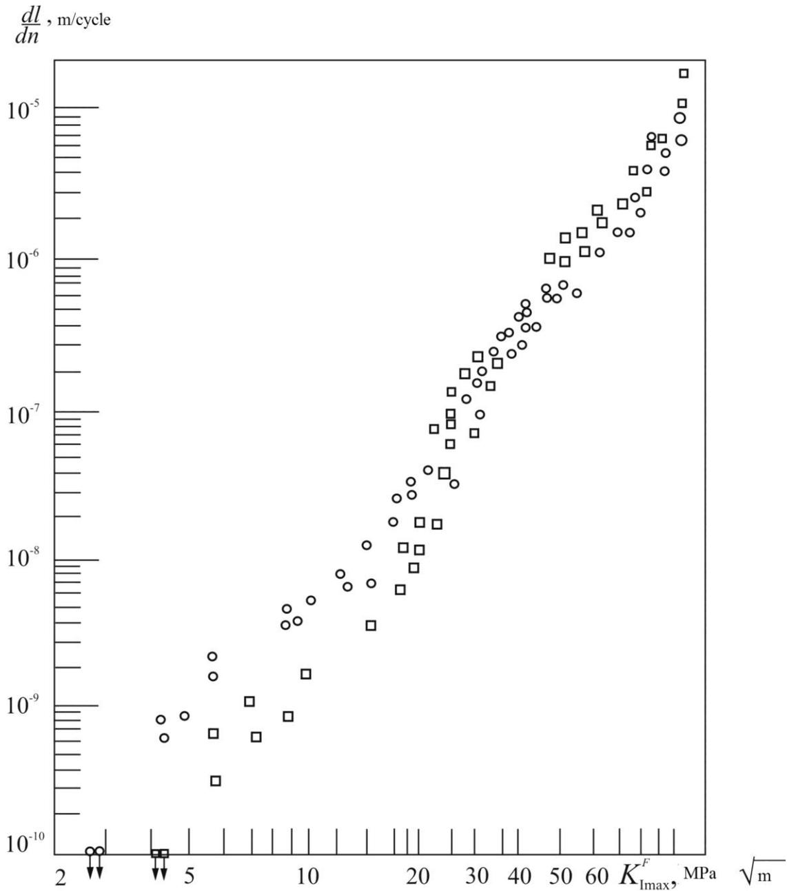
Fig. 1 - Experimental diagram «SIF - growth rate of a fatigue crack» for 08X18H12T steel after 100 thousand hours of operation time for specimens with CFD in a direction:  $\circ$  - circumferential,  $\square$  - axial
