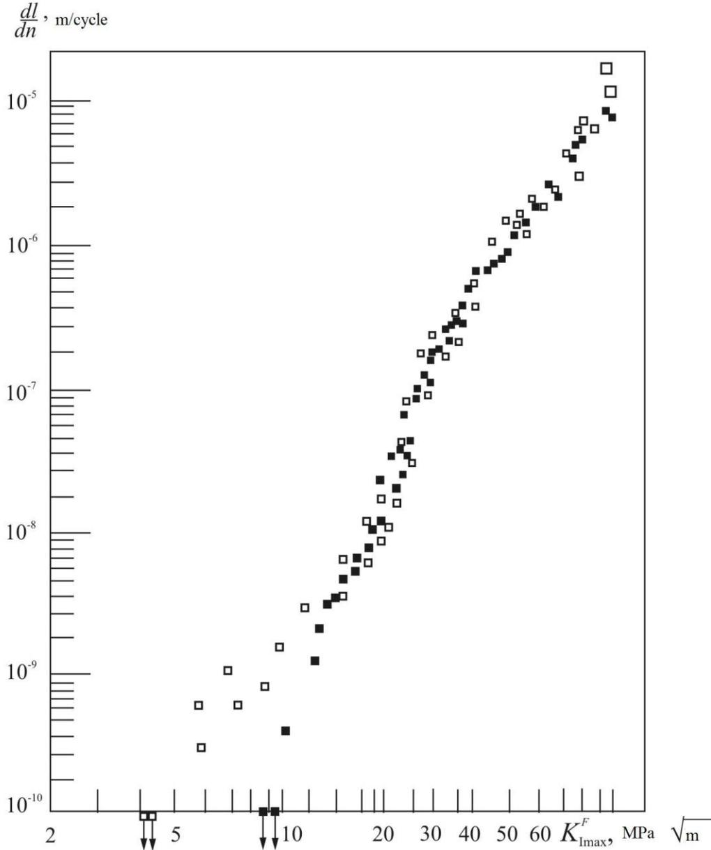
Fig. 2 - Experimental diagram «SIF - growth rate of a fatigue crack» for 08X18H12T steel depending on an operation time with CFD in an axial direction: ■ - an initial condition, □ - after 100 thousand hours of operation
