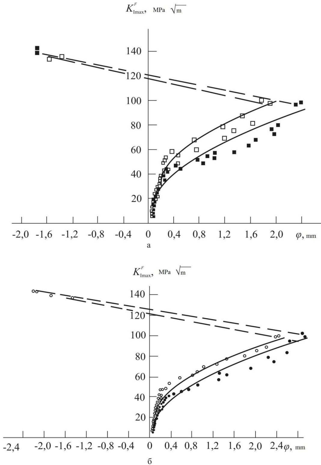
Fig. 3. - Diagram  $K_{\text{Imax}}^F - \varphi$  for specimens of 08X18H12T steel depending on an operation time with CFD in a direction: ● - circumferential, ■ - axial in an initial condition (a) and ○ - circumferential, □ - axial after an operational operating time (b)
