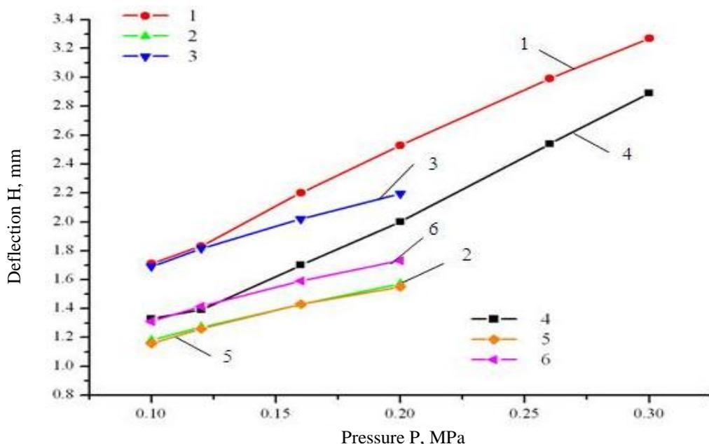
Fig. 4. Dependence of a deflection of H from pressure of P: 1—sample previously the deformed; 2 and 3 – calculation at  $E=2.1 \cdot 10^5$  MPa and  $E=8.577 \cdot 10^4$  MPa; 4—not deformed sample; 5 and 6 – calculation at  $E=2.1 \cdot 10^5$  MPa and  $E=1.573 \cdot 10^5$  MPa
