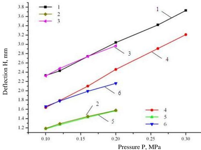
Fig. 3. Dependence of a deflection of H from pressure of P: 1–sample not deformable; 2 and 3 – calculation at  $E = 2.1 \cdot 10^5$  MPa and  $E = 3.756 \cdot 10^4$  MPa; 4–sample previously the deformed; 5 and 6 – calculation at  $E = 2.1 \cdot 10^5$  MPa and  $E = 8.981 \cdot 10^4$  MPa
