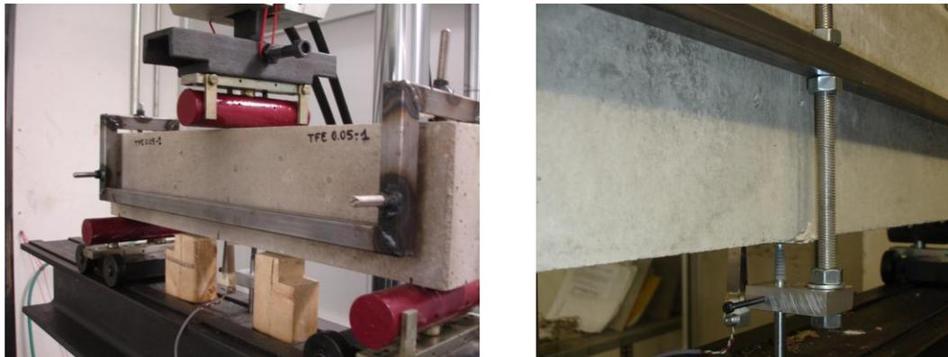
Fig.5. Three-point bend test of the TFE05 specimens (left) and its instrumentation (right)
