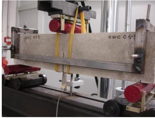
Fig.6. Three-point bend test of SWC05 specimens with weight compensation
