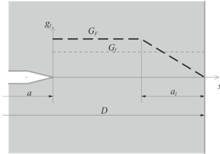
Fig.1. Local fracture energy model of Hu et al.
