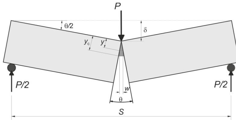
Fig.2. Rigid-body model of the behavior of the specimen at the end of the test.
