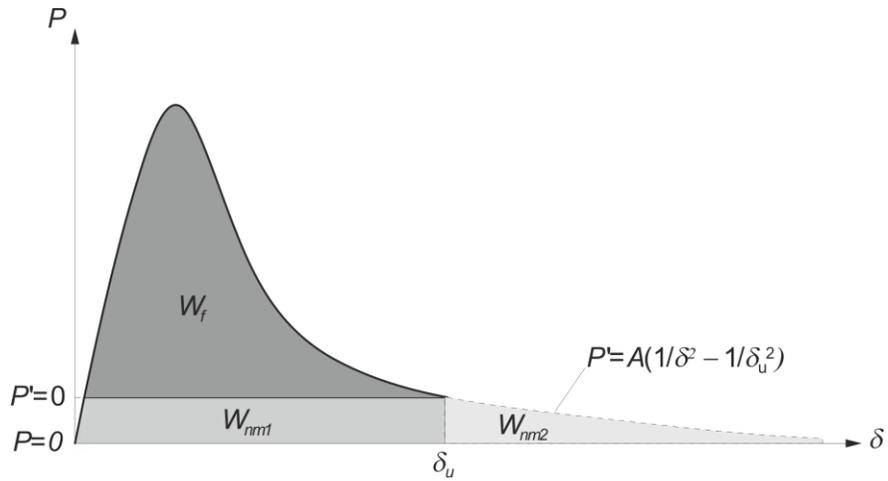
Fig.3.  $P$ - $\delta$  curve in a three-point bend test and the measured ( $W_f$ ) and non-measured ( $W_{nm1}+W_{nm2}$ ) fracture energy.
