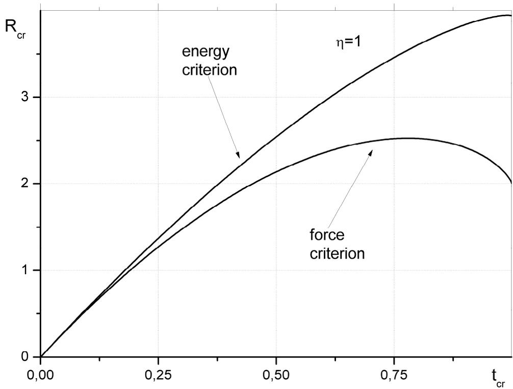
Fig.2. Dependence of  $R_{cr}$  on the relative bridged zone size, the criterion comparison,  $\eta = 1$ .
