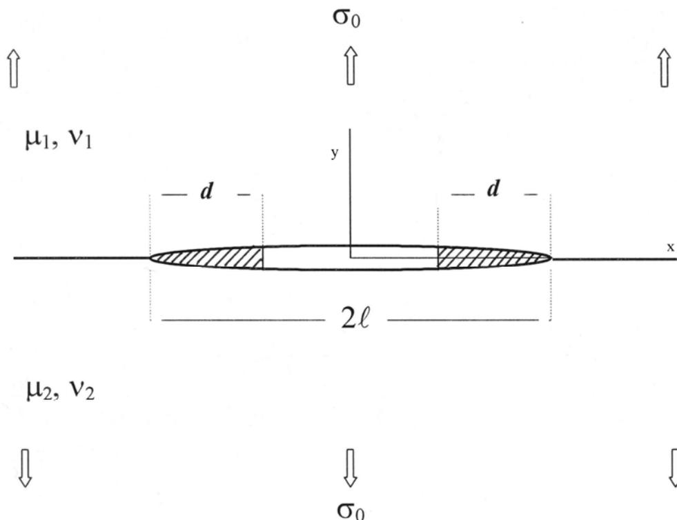
Fig. 1. Bi-material plate with bridged interface crack.
