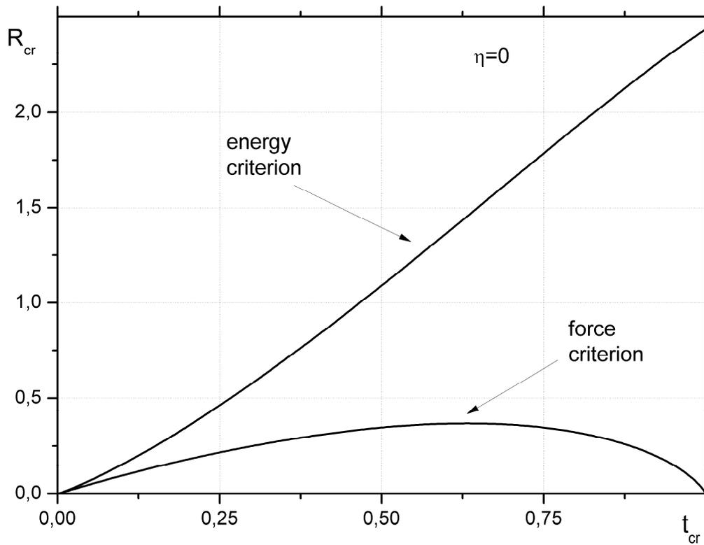
Fig.3. Dependence of  $R_{cr}$  on the relative bridged zone size, the criterion comparison,  $\eta = 0$ .
