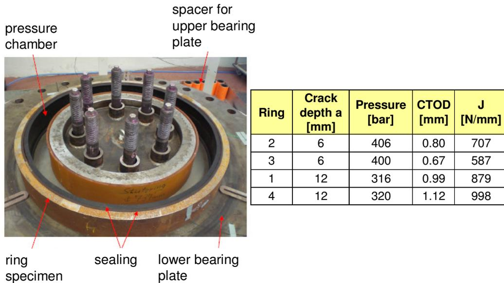
Fig. 4: Ring expansion test set-up (left), major test results (right)
