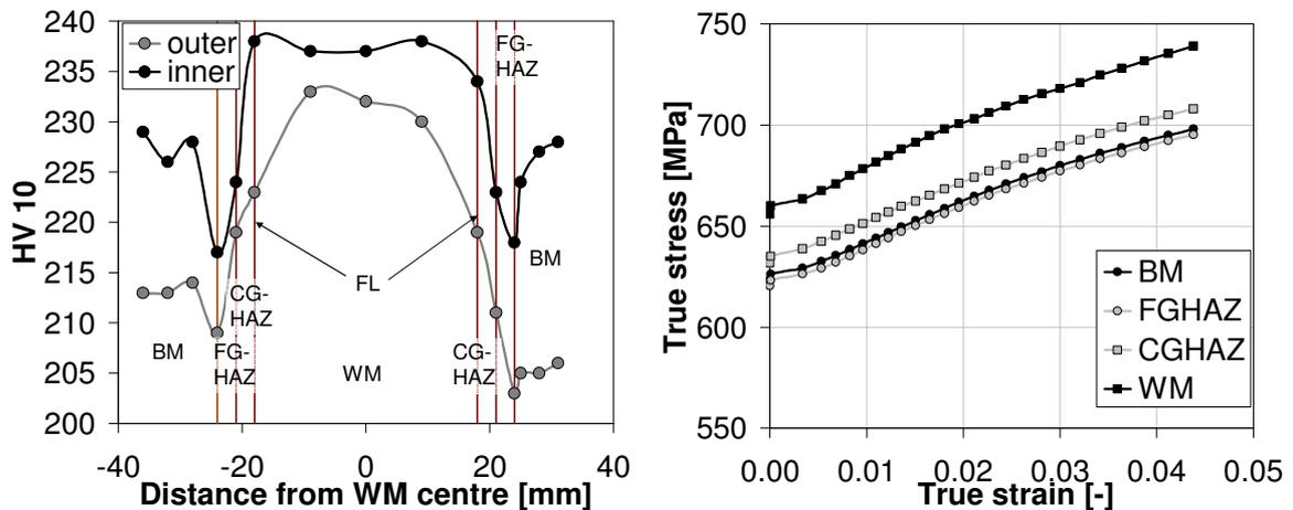
Fig. 3: Hardness values HV10 of X80 weld (left), true stress-strain curves (right)
