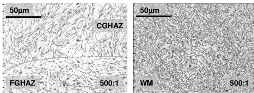
**Fig. 2:** Microstructure of HAZ and WM
