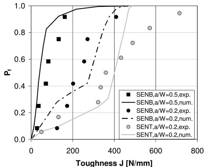
Fig. 6: Experimental and predicted  $P_f$ -values for SENB and SENT specimens
