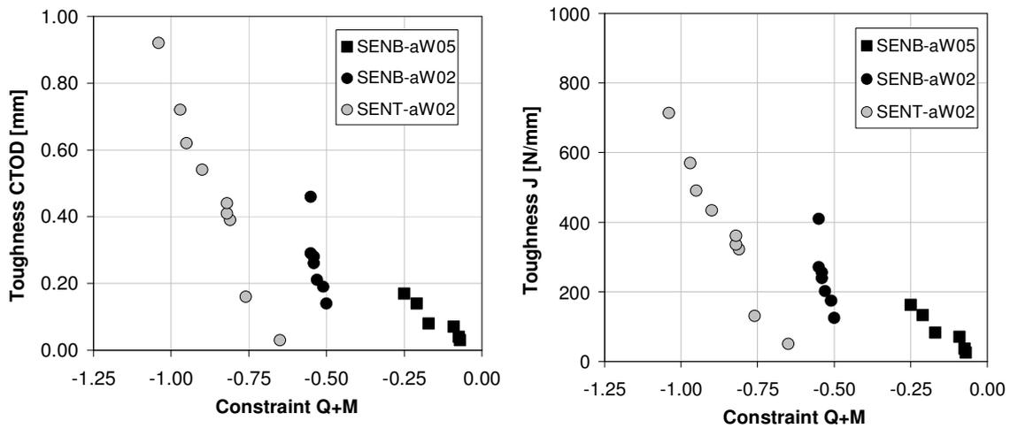
Fig. 5: CTOD (left) and J (right) toughness values vs. constraint Q+M
