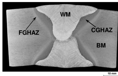
**Fig. 1:** Macrograph of weld cross section
