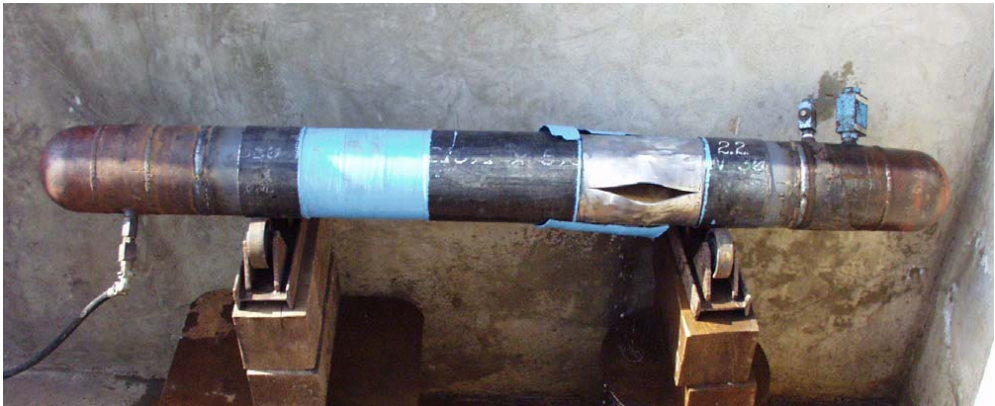
Figure 4. Steel pipeline section repaired with carbon fibre reinforced polymer matrix composite, after burst test (see Table 3., B_b7 pipe section).
