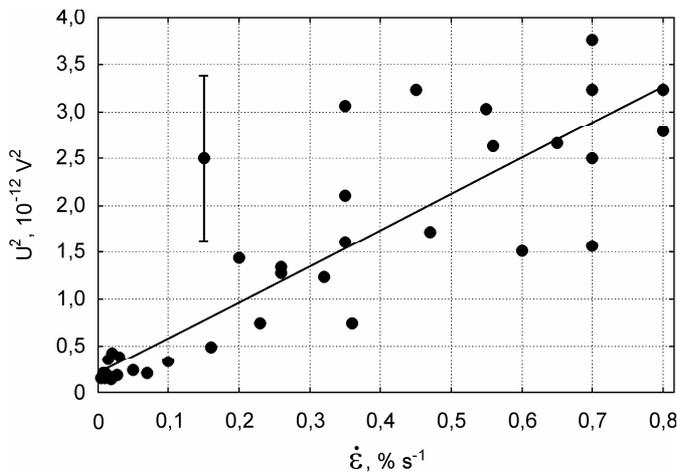
Fig. 4. The dependence of the square of acoustic signal amplitude on the velocity of deformation at jumplike section. The linear approximation of the dependence is made at the correlation coefficient 0.9.
