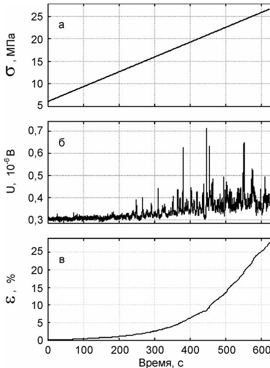
Fig. 2 Acoustic emission and deformation in the first isothermic ( $T=600^{\circ}\text{C}$ ) thermomechanical cycle: a) linear increase of mechanical stress in the cycle; б) the dependence of root-mean stress of acoustic emission on the duration of loading in the cycle; в) the dependence of deformation on the duration of loading in the cycle.
