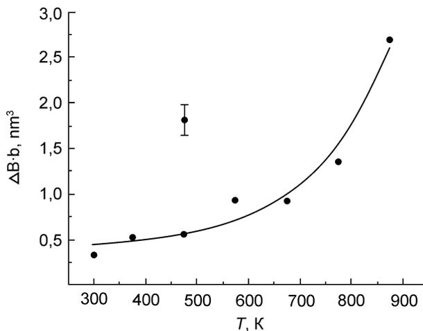
Fig. 3 The dependence of activation volume of elementary deformation act in Al on the temperature of thermomechanical cycle.
