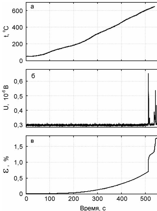
Fig. 1 Monotonous and jumplike nature of deformation accumulation and impulsive nature of acoustic emission in thermomechanical cycles at a mechanical stress of about 18 MPa: a) the dependence of temperature on the process duration; б) the dependence of root-mean stress of acoustic emission on the duration of heating; в) the dependence of deformation on the duration of heating.
