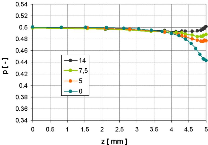
Fig.6. Variation of the stress singularity exponent along crack front for different crack front angles  $\alpha$ . Material properties is corresponds to PMMA (Poisson's ratio is 0.365).
