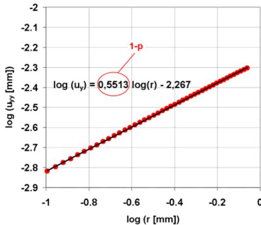
Fig.1. Typical example of displacement regression of the stress singularity exponent in 3D body
