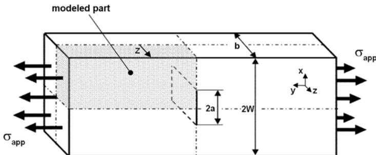
Fig.2. Model used for finite element calculations
