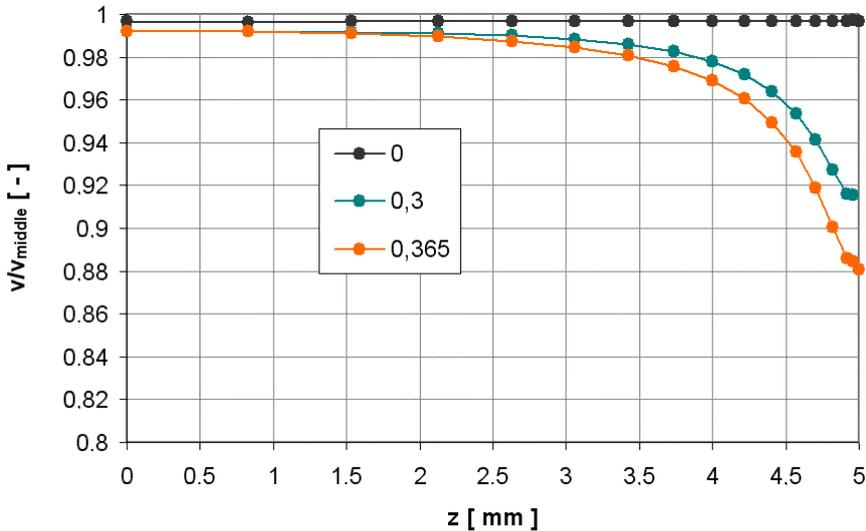
Fig.4. Variation of ratio between real fatigue crack propagation rate  $v$  and FCPR in the middle of the specimen  $v_{middle}$  along the crack front for three Poisson's ratios.
