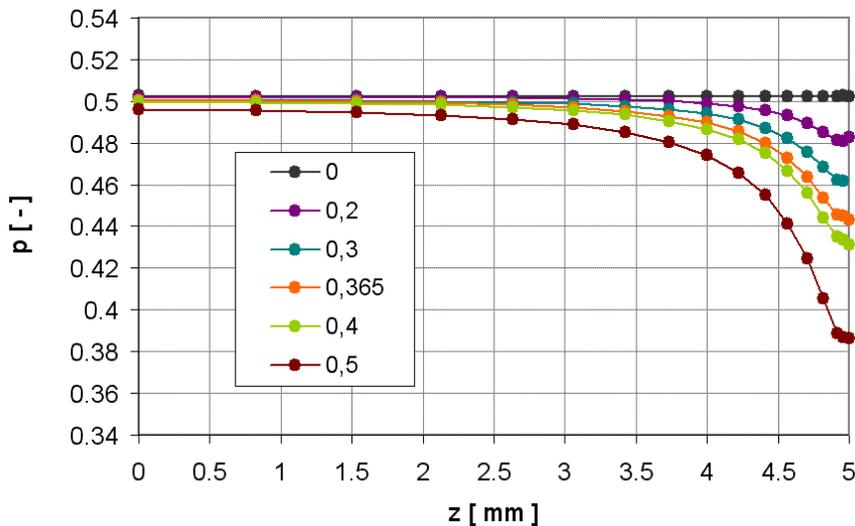
Fig.3. Variation of stress singularity exponent along the crack front for different Poisson's ratios.
