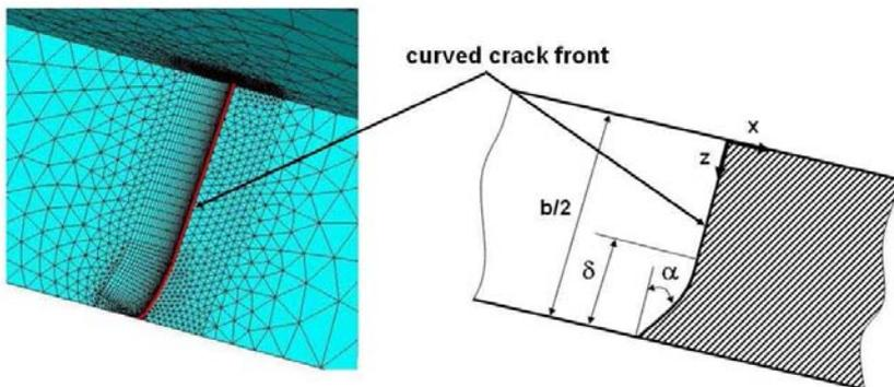
Fig.5. Example of the finite element mesh close to curved crack front and schematic description of the MT specimen cross section area.
