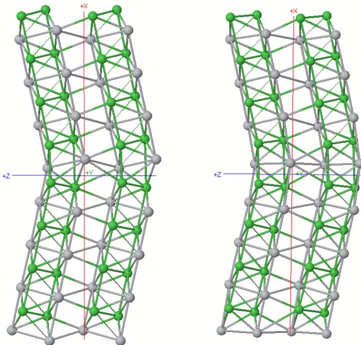
Figure 4: The super-cell containing twins in  $\{100\}$  planes before optimization of ionic position at the interface (on the left) and after the optimization (on the right).
