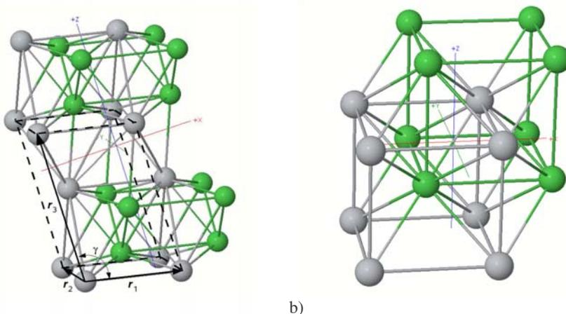
Figure 1. Two stable structures of NiTi alloy: a) martensite of monoclinic symmetry (with translational vectors  $r_1$ ,  $r_2$  and  $r_3$ ) and b) cubic austenite.
