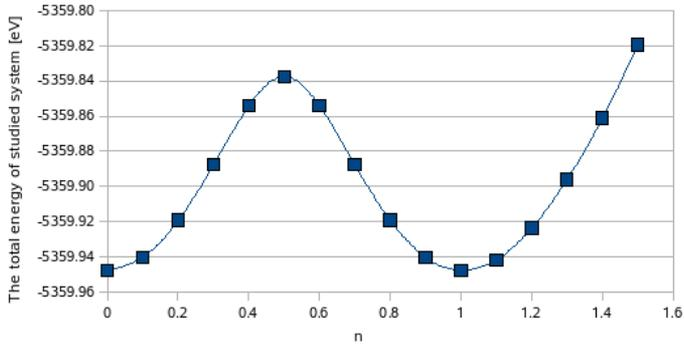
Figure 3: The total energy  $E_{tot}$  as a function of normalized tilt  $n$  where  $n = 0$  for B19' martensite and  $n = 1$  at the state corresponding to the tilted B19' martensite.
