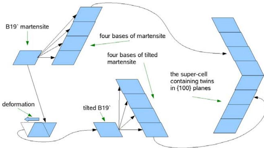
Figure 2: The process of building the computational super-cell containing  $\{100\}$  twins.
