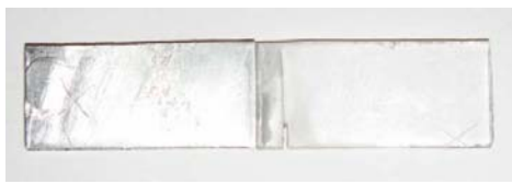
b. Bimaterial Aluminum - PMMA crack path
