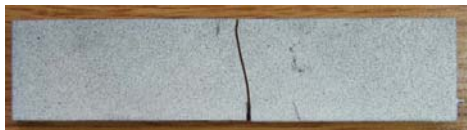
a. Homogeneous PMMA crack path
