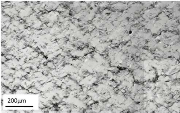
Fig. 5: Extract of the surface scan taken after 18,000 load cycles
