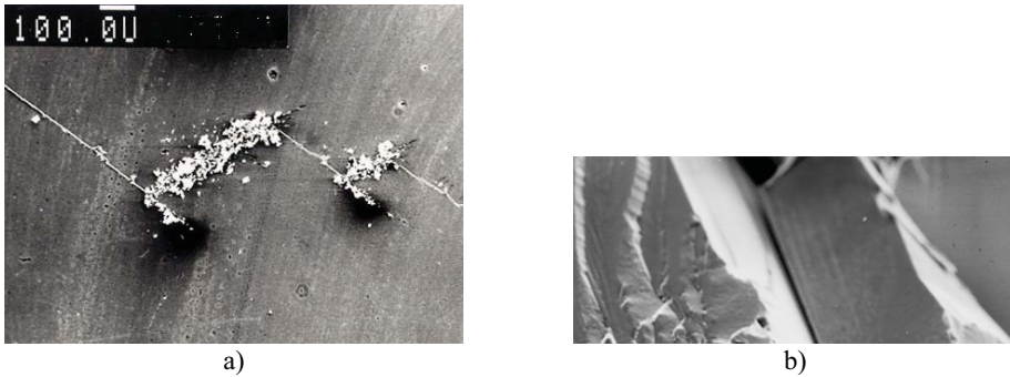
Figure 3. Zig-zag stage I crack grown in high vacuum ( R=-1 and 35Hz) in an Al-Zn-Mg singlecrystal not oriented for easy slip: a) crack profile with evidences of crack closure, and b) crystallographic crack surface.
