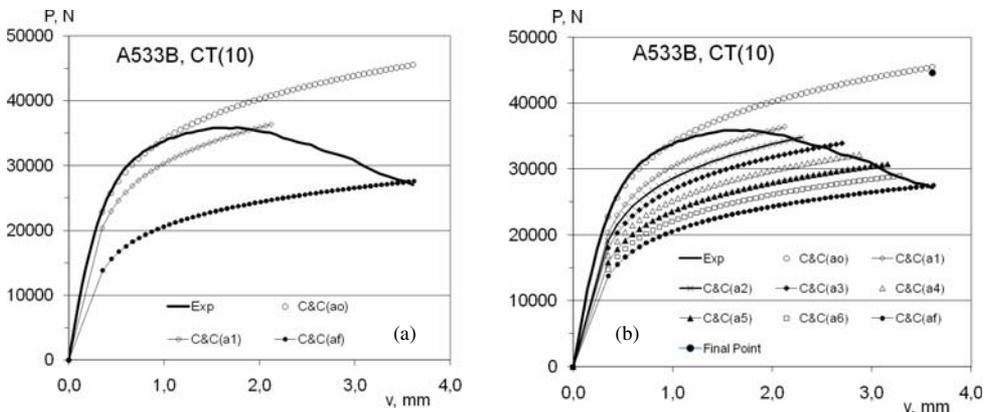
Figure 2.-  $P$ - $v$  plots of the A 533B 1-T C(T) specimen with  $a_o/W = 0.6$ . On the left, the experimental curve with three  $a$  constant curves; on the right, six intercept  $a$  constant curves.
