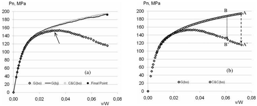
Figure 3.- Normalized  $P$ - $v$  data to show the corrected force method.
