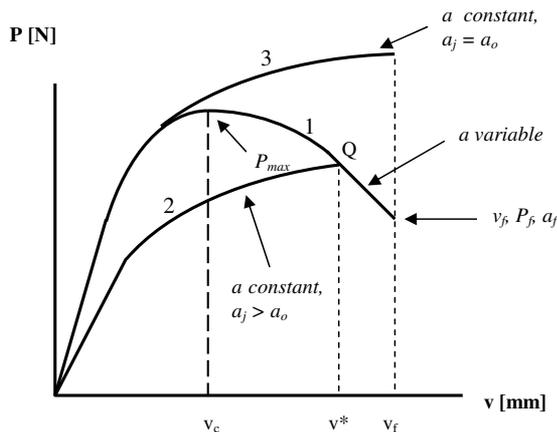
Figure 1.- Schematic force-displacement curves for variable and constant crack size.
