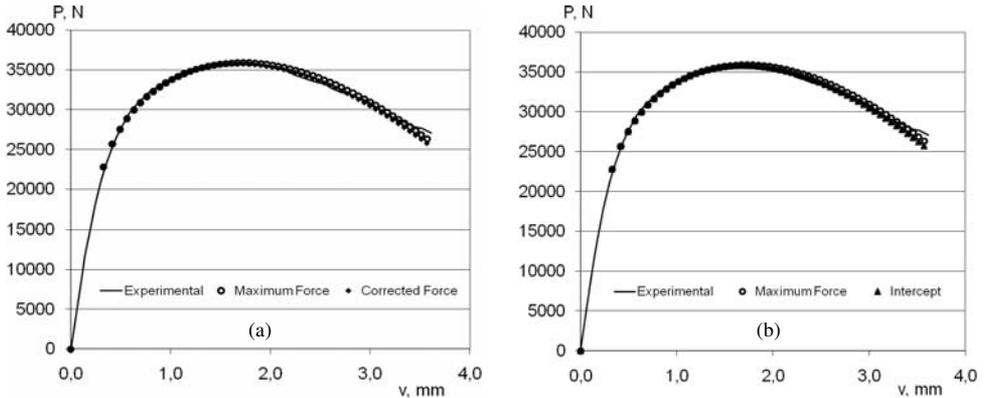
Figure 5.- DZL model curves constructed with the crack growth law parameters obtained from *maximum force* and *corrected force* (left) and *maximum force* and *intercept* methods (right).
