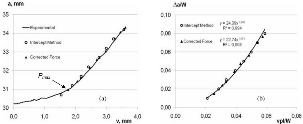
Figure 4.- Results of the intercept and corrected force methods, shown against experimental data (left). On the right, the crack growth law plot for the intercept and corrected force methods.
