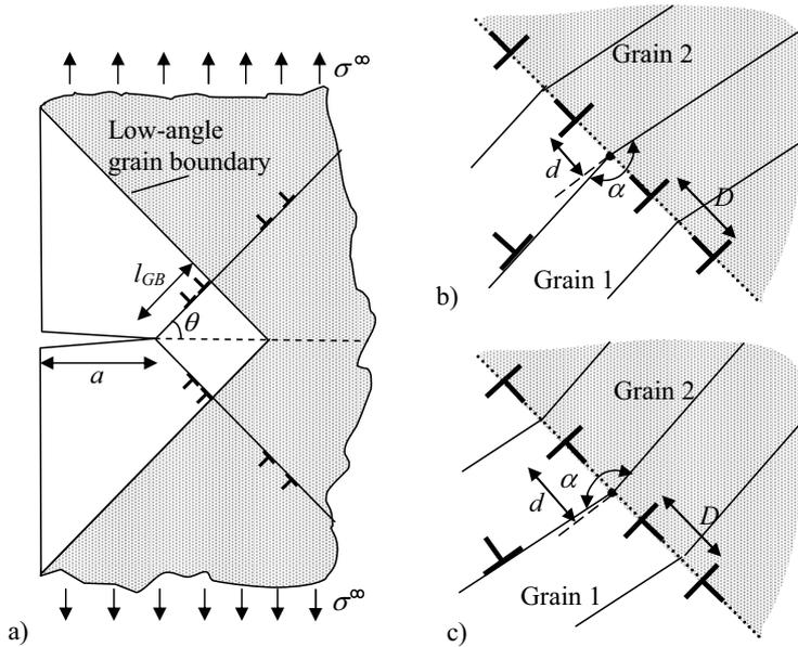
Figure 1. a) Geometry and loading of the edge crack, and the dislocation arrangement in b) a positive and c) a negative low-angle grain boundary, respectively.
