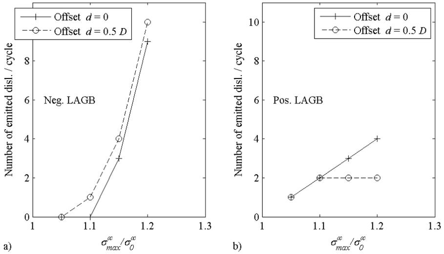
Figure 2. Crack growth rates vs maximum load in a cycle for  $l_{GB}=a_0/8$  with a) a negative and b) a positive low-angle grain boundary, respectively. Results for two offset distances  $d$  are shown.
