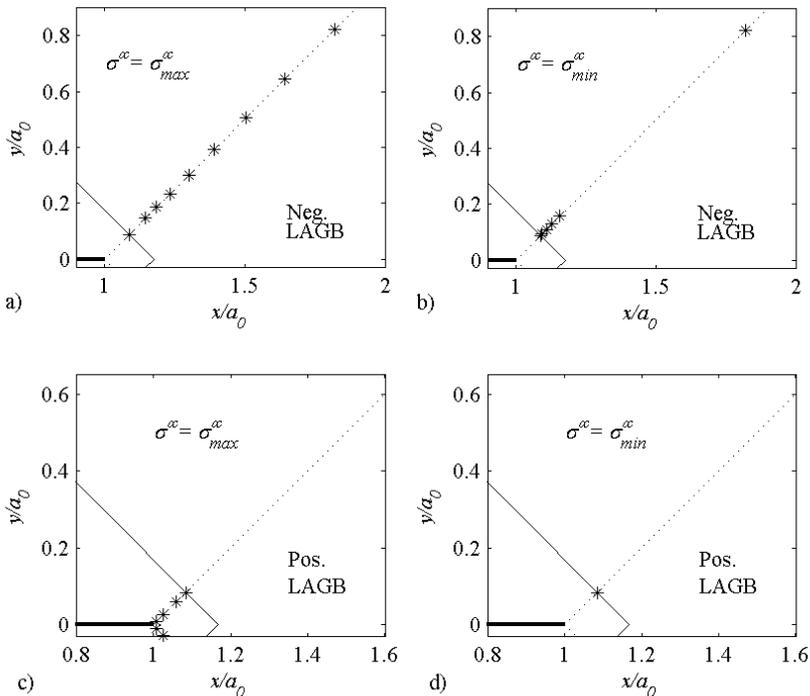
Figure 3. Dislocation distribution at a) maximum load and b) minimum load, for a negative LAGB, and c) maximum load and d) minimum load, for a positive LAGB. For all cases  $\sigma_{max}^{\infty}=1.15\sigma_0^{\infty}$ ,  $l_{GB}=a_0/8$ , and  $d=0$ .
