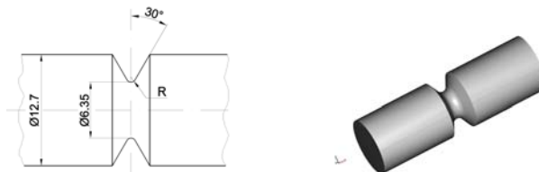
Fig. 4. Geometry of a round notched specimen, where R=0.529 mm ( K_t=2.8 ) or R=1.588 mm ( K_t=1.8 ) from [15].
