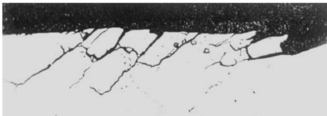
Fig. 9. Crumbling of the roller surface from the rail steel under contact fatigue testing [19].
