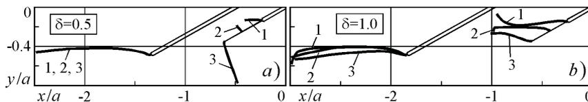
Fig. 6. Propagation paths of two non-equal parallel cracks depending on the first crack length;  $f = 0.1$ ;  $\epsilon_2 = l_2/a = 1.0$ ;
