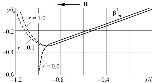
Fig. 3. Crack growth paths versus parameter  $r$  of the pressure intensity on its faces;  $\beta = 20^\circ$ ,  $f = 0.1$ ,  $\varepsilon = l_0/a = 0.43$ .
