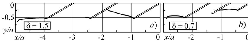
Fig. 8. Propagation paths of three equal (a) and non-equal (b) cracks:
