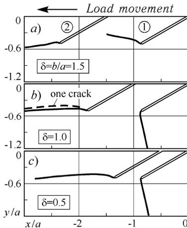
Fig. 5. Propagation paths of two equal parallel cracks depending on distance  $\delta$  between them;  $f = 0.1$ ;  $\varepsilon = l/a = 1.0$ .
