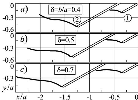
Fig. 7. Propagation paths of two non-equal cracks depending on the distance between them;
