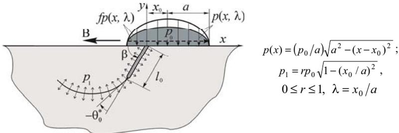
Fig. 2. A calculation model. **B** is the direction of the counterbody motion;  $f$  is the friction coefficient.
