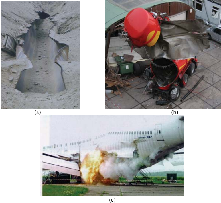
Figure 1 (a) full scale burst test of gas pipeline [1]; (b) explosion of a road tanker (2008); (c) explosion of airplane (DERA test, 2001).
