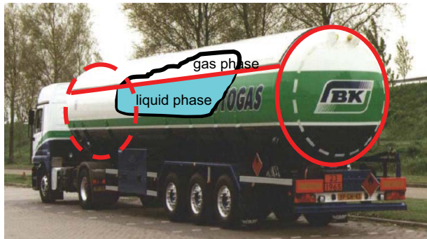
Figure 8 Representative LPG tank, with cohesive zones (red lines).
