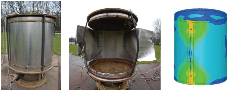
Figure 6 Failure of a pressurized aluminium barrel. (left) setup with measuring devices, (middle) barrel after explosion; (right) FE model, stress field during crack propagation.
