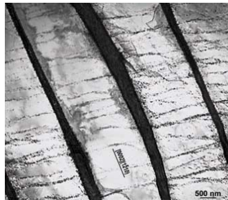
Figure 10. Dislocations structures after creep during 7 000 hours at \sigma_{max} / \sigma_y = 1 .
