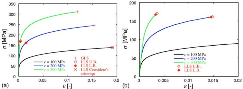
Figure 5: (a) Simulated composite stress-strain curves for different matrix strength coefficients, and failure as predicted for LLS and GLS. (b) Close-up at small strains for the LLS model. The symbols  $\diamond$ ,  $\blacklozenge$  denote abrupt failure, while  $+$  and  $\times$  denote failure by tensile instability. Power law matrix behaviour  $\sigma_m = c \epsilon_m^n$  ( $n = 0.2$ ,  $V_r = 0.5$ ,  $N = 10^7$ ,  $m = 3$ ,  $\sigma_0 = 700$ MPa).
