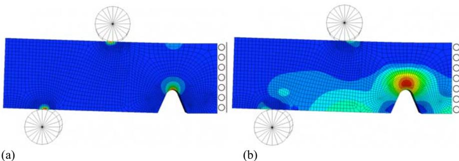
Figure 4: FEM computed fields of (a) the largest principal strain and (b) the largest principal stress in the centre plane of a double notched bend bar (3D computation).
