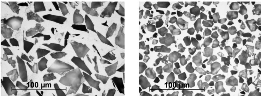
Figure 1: Optical micrographs of PRMMCs with (a) 35  $\mu m$  angular and (b) 25  $\mu m$  polygonal  $Al_2O_3$  reinforcements (dark phase).
