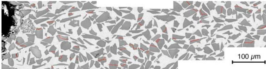
Figure 3: Metallographic cut of an unbroken notch in a double notched bend bar (in the centre plane of the specimen). Metallographically visible particle cracks are highlighted with red lines.
