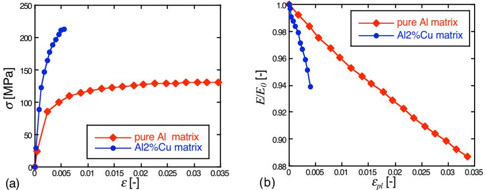
Figure 2: Pure aluminium and Al-2%Cu alloy reinforced with angular 35 micron alumina particles. (a) Typical true stress-strain curves, and (b) evolution of Young's modulus (normalized by its initial value) as a function of plastic strain. Failure of the pure aluminium matrix composite occurs following Considere's criterion, whereas the stronger alloyed materials fail before.
