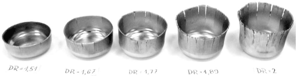
Fig. 8 Delayed cracking after deep drawing test in cups with different drawing ratios.
