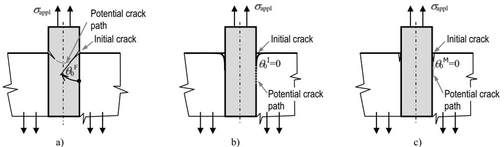
Fig. 3 Damage eventualities of fibre-matrix system in the case of pulled-out fibre (e.g. while crack bridging) a) rupture of fibre, b) interfacial crack, c) crack in the matrix (crack direction parallel to the interface)
