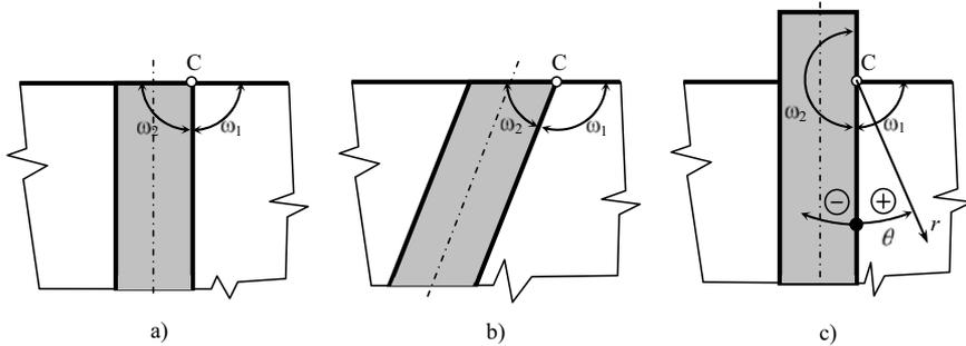
Fig. 1 Possible configurations of the fibre-matrix intersection at a surface considered in the paper. Polar coordinates ( $r, \theta$ ) with sign convention of the direction of crack initiation.
