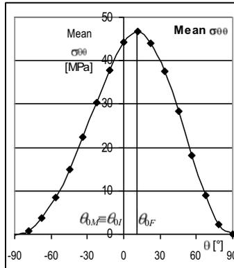
Fig. 2 Numerical analyses of the mean value of the tangential stress around the free fibre ending in the plane of surface.
