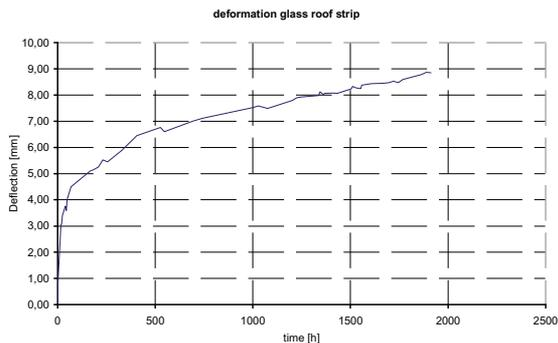
Fig. 11: Deflection-time diagram of 15 m roof strip
