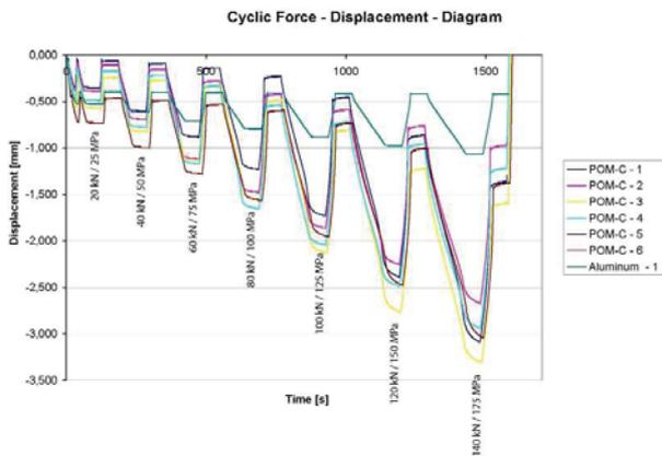
Fig. 8: Stress-strain diagram under cyclic force
