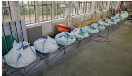
Fig 10a - 10b: Pane offset and creeping testing of 15 m roof strip with 1.20 kN/m<sup>2</sup>
