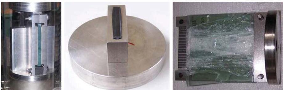
Figures 6a - 6c. Testing facility and deformed POM-C wedges in socket and failed glazing
