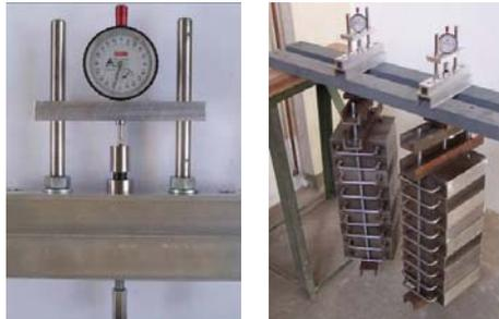
Fig. 9a - 9b: Testing facility for creeping
