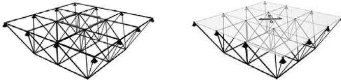
Fig. 2a and 2b: Compression elements in the upper layer of a traditional and a transparent space grid structures (half-octahedron plus tetrahedron)
