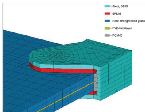
Fig. 7: FE-model of the node
