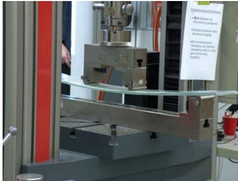
Figure 1 : Test set-up with glass specimens lying
