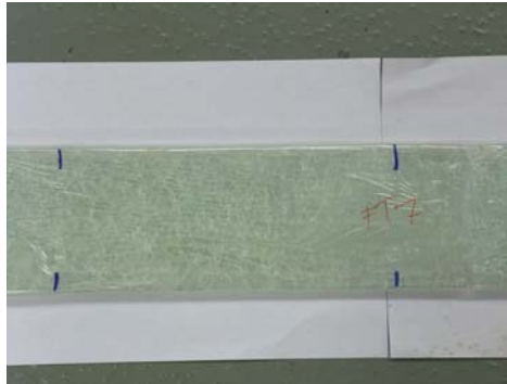
Figure 7: Failure pattern of fully tempered glass tested lying, failing at 107.7 MPa
