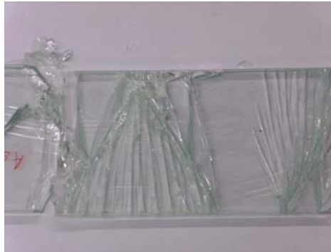
Figure 3: Failure pattern of annealed glass tested lying, failing at 55.8 MPa
