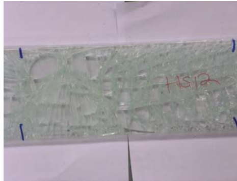
Figure 5: Failure pattern of heat strengthened glass tested lying, failing at 111.7 MPa
