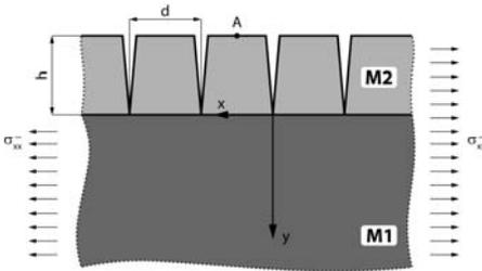
Figure 1a: Scheme of an array of periodically distributed edge cracks
