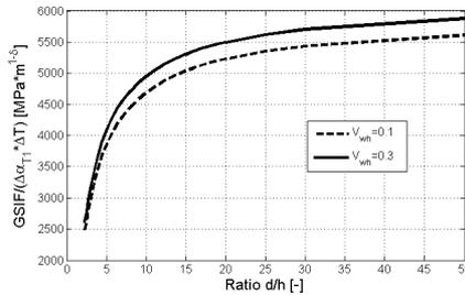
Figure 2b: GSIF normalized by the stress-free misfit strain  $\Delta\alpha_{T1}\Delta T$  as a function of the spacing/layer thickness ratio  $d/h$
