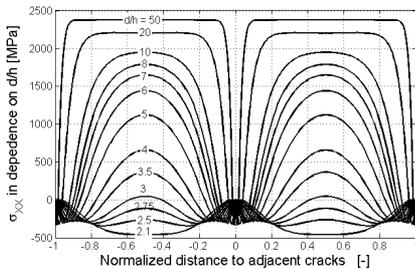
Figure 2a: Distributions of the normal stress component  $\sigma_{xx}$  between edge cracks for different spacing/layer thickness ratio  $d/h$ ,  $V_f = 0.3$ .
