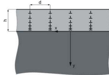
Figure 1b: Scheme of periodically distributed dislocation arrays
