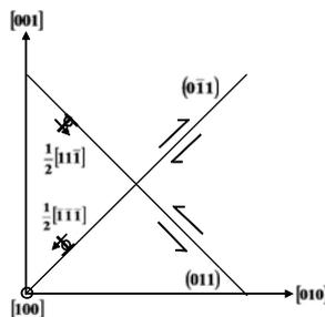
Fig. 1. Dislocations, relative to crystallographic axes. The slip planes are viewed edge on. Shear stresses are shown for an equivalent applied tensile stress along [001]. The Burgers vectors are foreshortened in this view.
