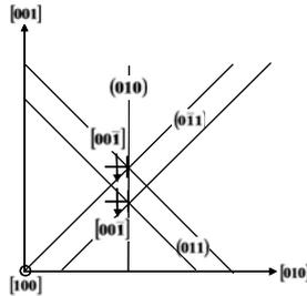
Fig. 2. Formation of sessile edge dislocations on (010) plane. Each dislocation results from the combination of two glide dislocations shown in Fig. 1.
