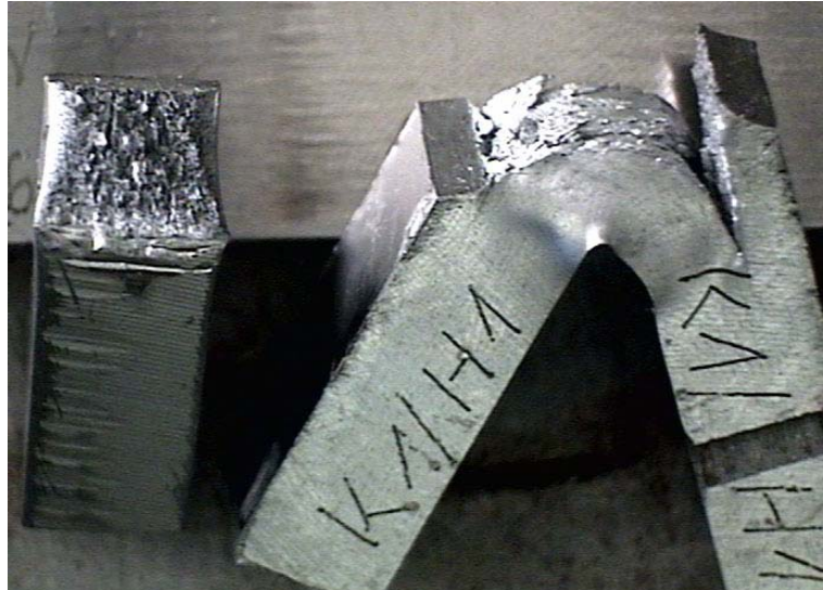
FIGURE 2. Typical appearance of the fracture of specimens cut from the pipe being in service and subjected to the impact tests: (left) specimen from „top” section; (right) specimen from “bottom” section.
