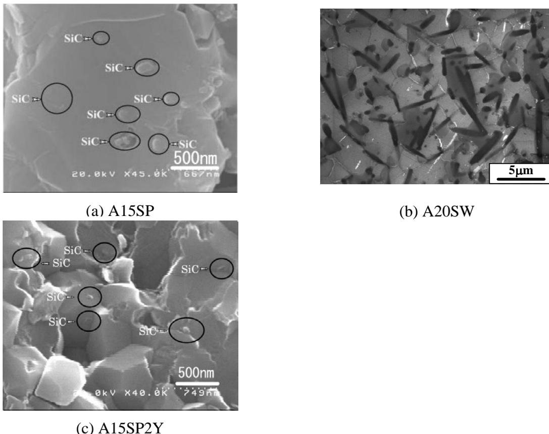
Fig. 2 Microstructure of (a) A15SP, (b) A20SW and (c) A15SP2Y
