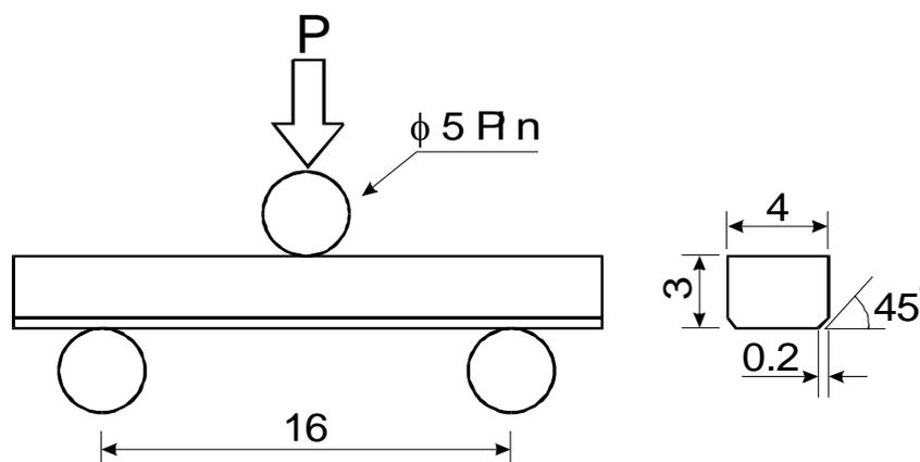
Fig. 1 Three point bending specimen and test system, dimensions in mm
