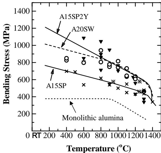
Fig. 4 Temperature dependence of the bending strength of (a) A15SP, (b) A20SW and (c) A15SP2Y crack-healed at 1300 °C for 1 h
