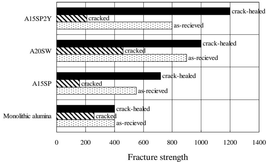
Fig. 3 shows the bending strength at RT of the as-received, cracked and crack-healed specimens, with the values of the monolithic alumina.
