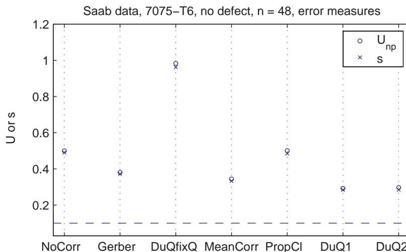
Figure 1. Error measures for one of the Saab specimen types. The broken line shows the estimated standard deviation due to inherent scatter.
