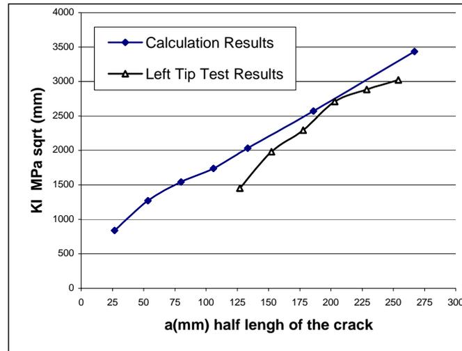
FIGURE 1. Comparison Between Current Analysis and Results Back Calculated from Experiment (Left Crack Tip).
